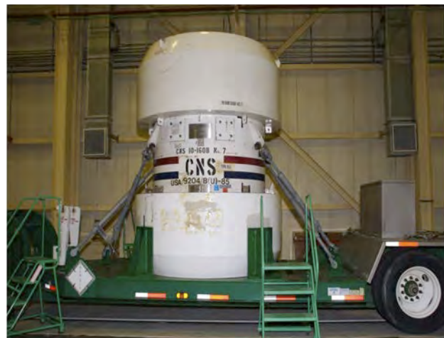
Figure 4 Type B Shipping Cask on Flatbed Trailer
