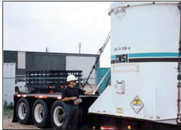
Figure 3 Type A Shipping Cask on Flatbed Trailer
