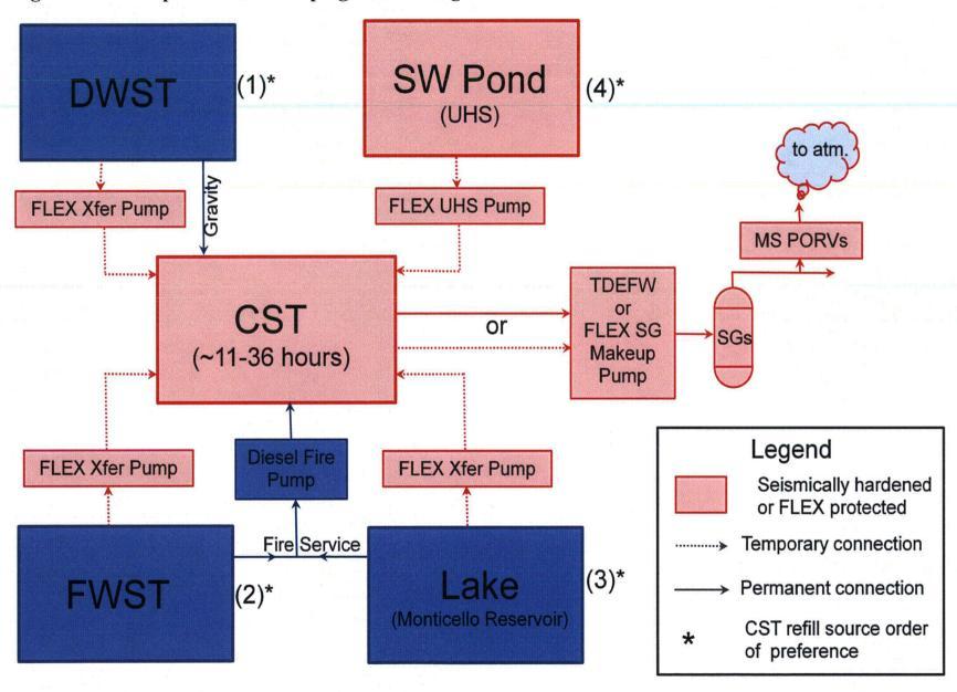
Figure 4 - Conceptual Strategy for Reactor Makeup and Reactivity Control
