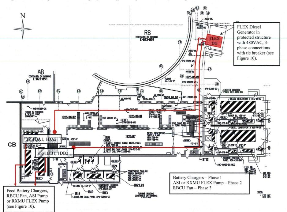
Figure 10 - Conceptual Coping Strategy to Repower RBCU Fan(s), Batteries, ASI/RXMU FLEX Pump
