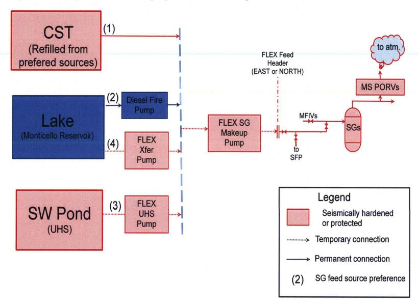
Figure 2 - Conceptual Diverse Strategy for Supplying the FLEX Feed Header
