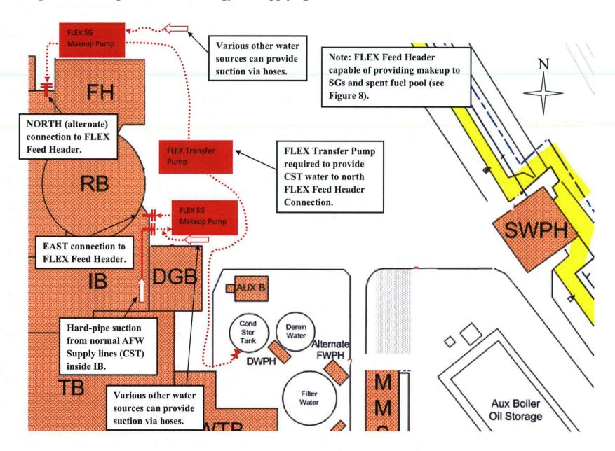
Figure 3 – Conceptual Phase 2 Coping for Refilling of CST
