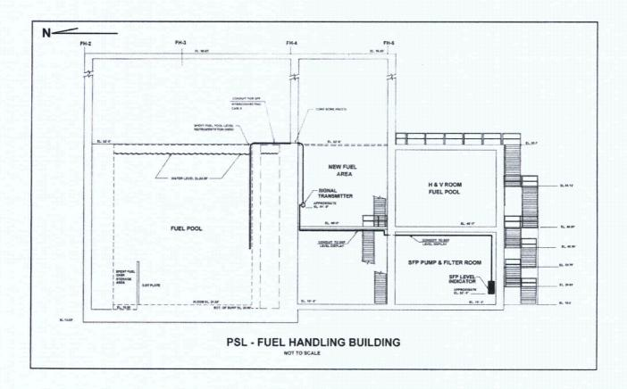
As shown, the signal transmitter for each channel is located outside the SFP room, one floor elevation lower in the new fuel storage area. The level indicator enclosures, including independent UPS and backup batteries for each channel, are located on the ground floor of the SFP pump and filter room (plant elevation 19.5').
