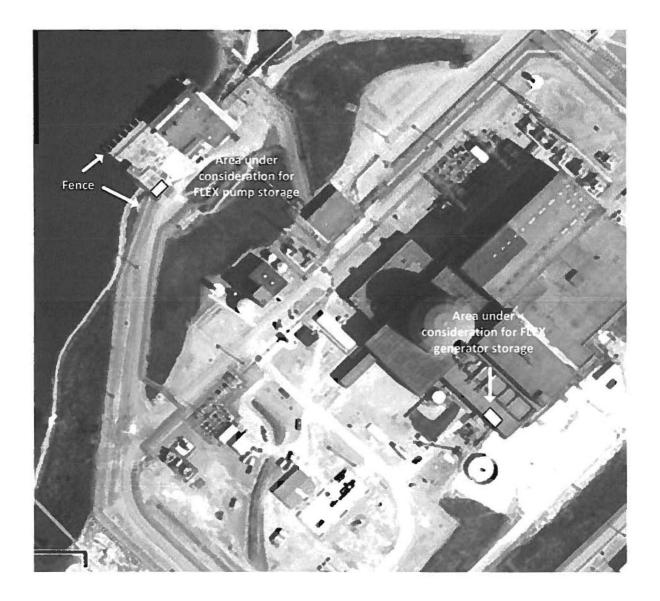
Figure 8 RRC Equipment Deployment Conceptual Sketch
