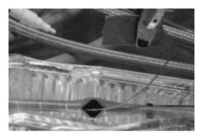
Figure 2-4 A wire probe is inserted into the fuel rod to measure the voided cladding length
