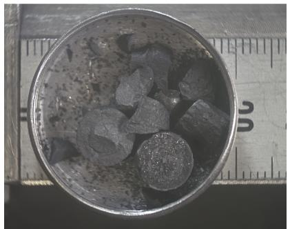
Figure 2-71 Fuel fragments collected from the bottom of rod 196 after gentle shaking just before gamma scan
