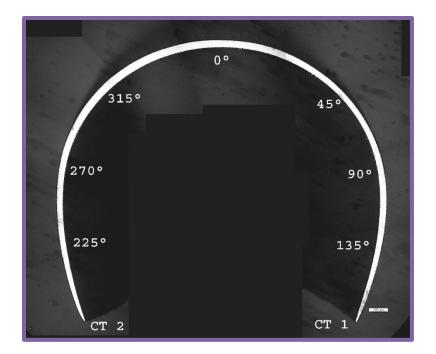
Figure 2-15 Macrograph of cross section from the rupture region of rodlet tested in LOCA Test 191
