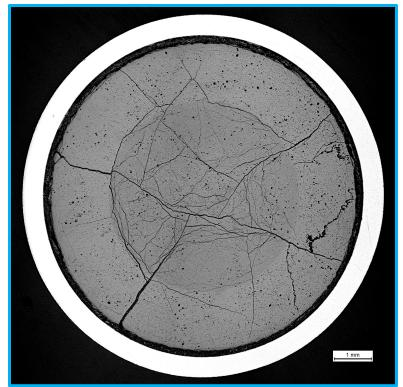
Figure 2-38 Macrograph of transverse cross section 35 mm from the bottom of the rodlet tested in LOCA Test 192
