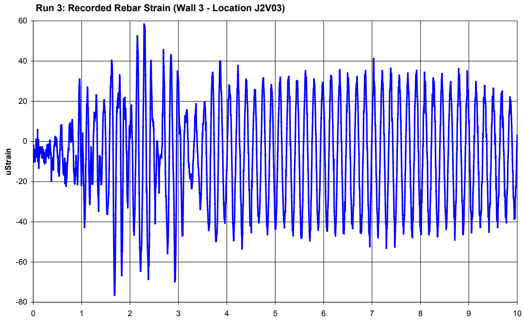
Figure 2-24 Rebar strain on Wall 3 recorded during RUN3 test
