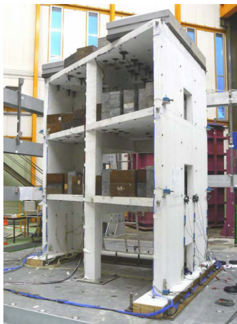
Figure 2-11 Instrumented and loaded SMART2008 structure on shaking table prior to the seismic tests
