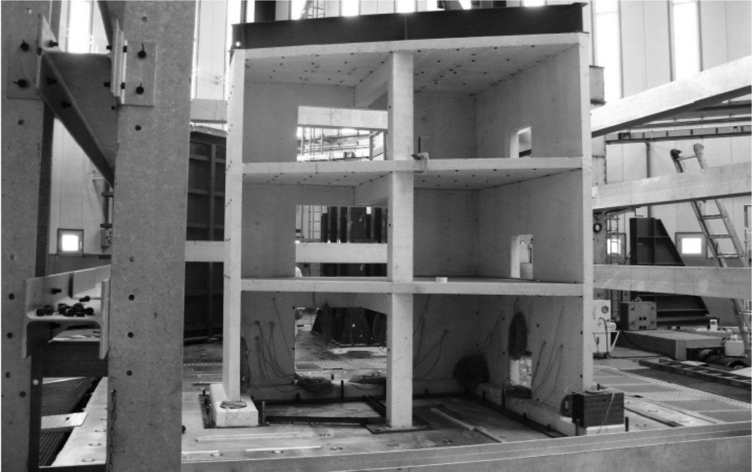
Figure 1-1 SMART2008 test structure on the Azalee shaking table at CEA Saclay, France
