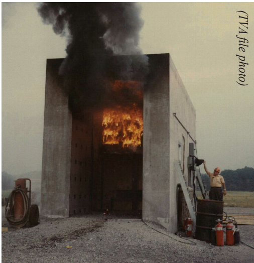
Picture of TVA Browns Ferry seal penetration tests
