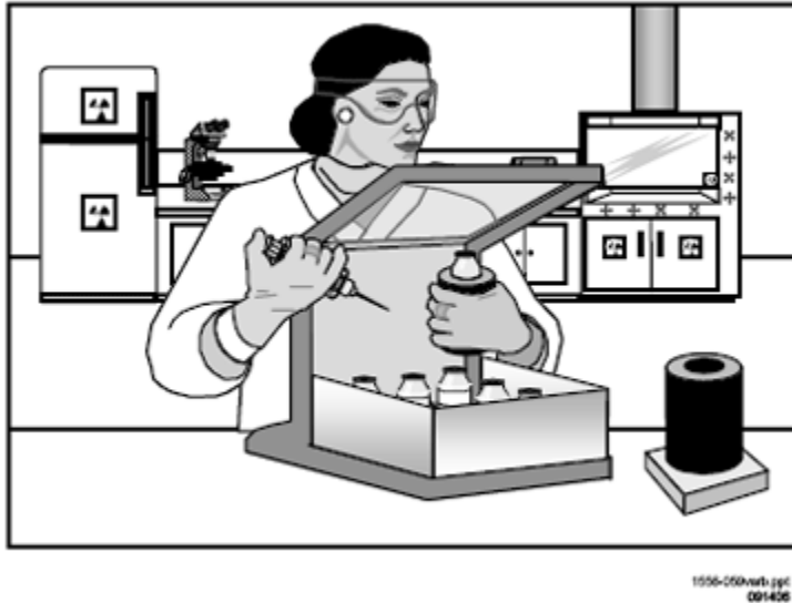
Figure 8.8 Use of Appropriate Shielding.
