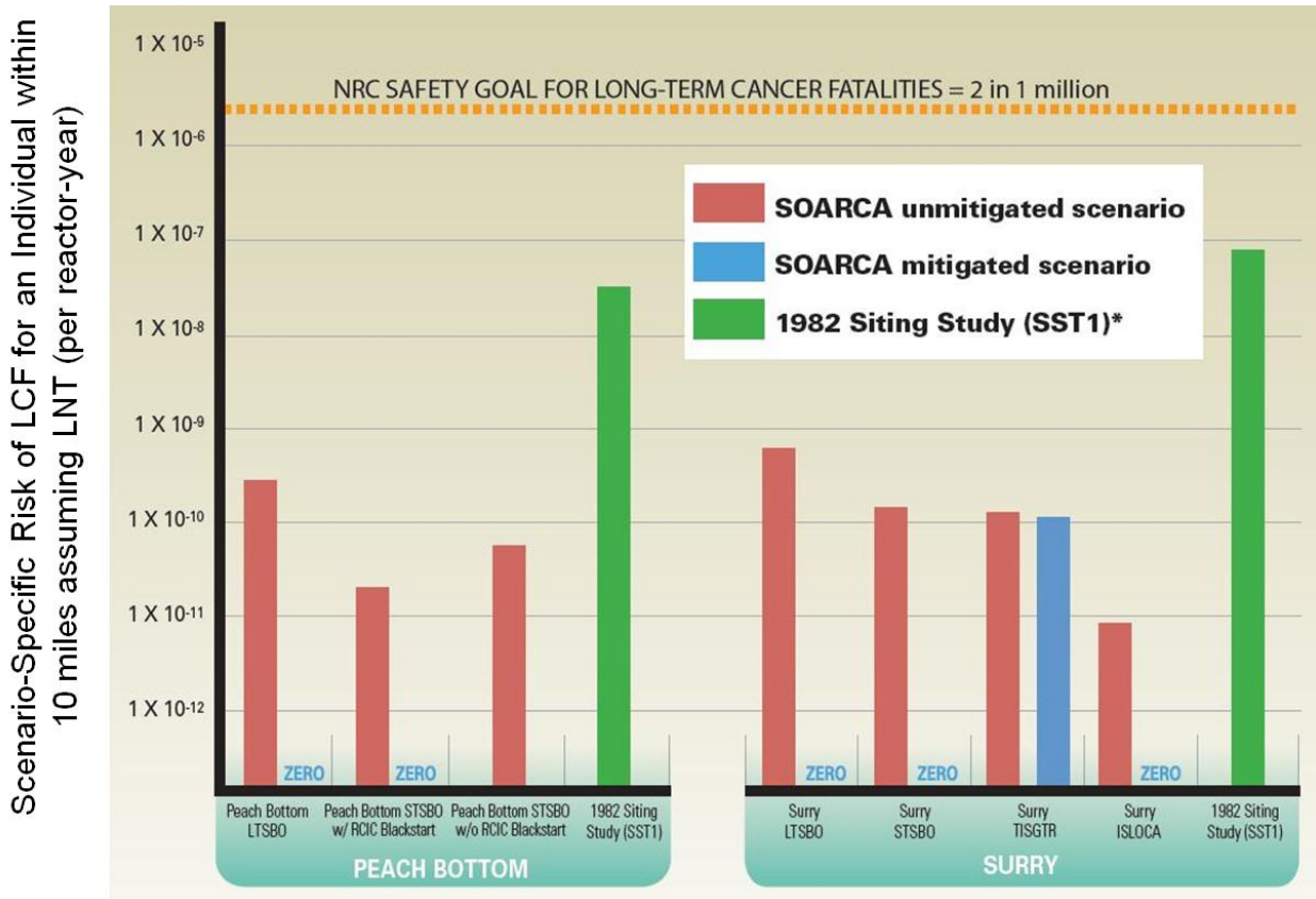
Figure ES-3 Comparison of individual LCF risk results for SOARCA mitigated and unmitigated scenarios to the NRC Safety Goal and to extrapolations of the 1982 Siting Study SST1 (plotted on logarithmic scale).
