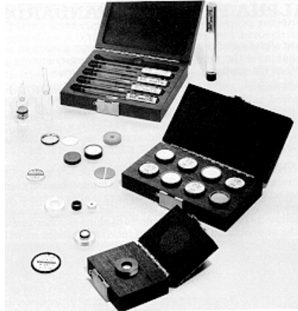
Figure 5.1 Calibration and Reference Sources. Calibration and reference sources may not need a registration by the NRC or Agreement States.
