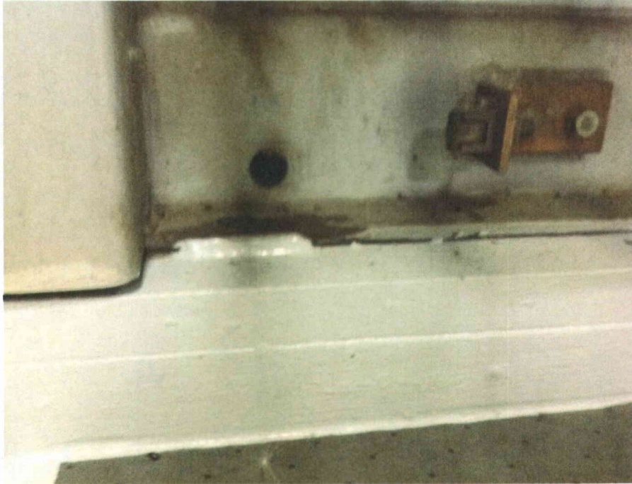
XDF1-2 Stitch Weld Front Unit is stitch welded along the entire front of the component
