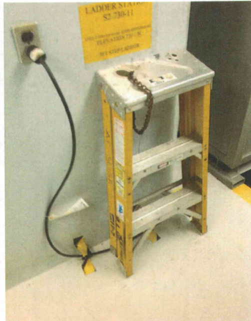
File Name: SWGR AE(5).jpg Description: Properly restrained ladder identified in the area
