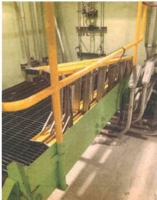
File Name: 1-60-3-3-29.jpeg Description: Ladder in the area identified to be properly restrained.
