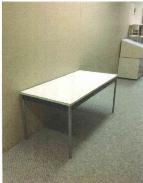
File Name: 1-68-1-1-03.jpeg Description: Table not restrained
