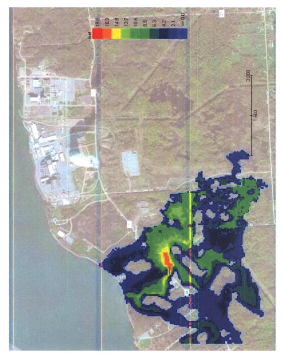
Figure 2.2-14: Grid Element Maximum Flow Depth
