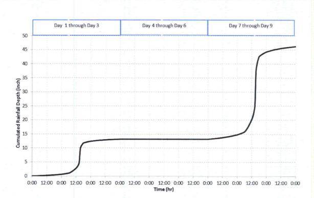
Figure 2.2-5: Input Hyetograph for 72-Hour PMP
