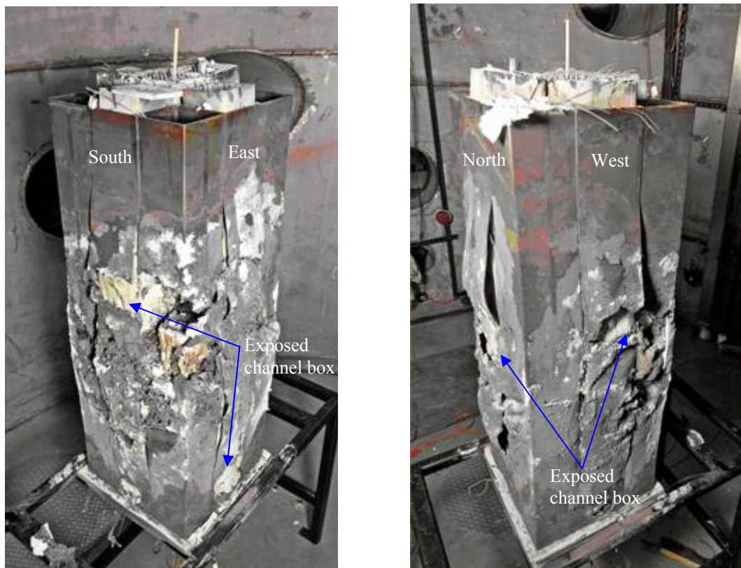
Figure 8.24 Post-ignition test photographs of the apparatus with the insulation removed
