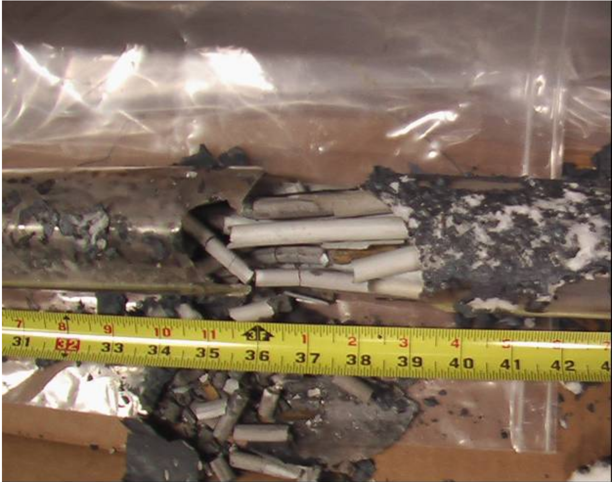
Figure 3.23 Detail of heater rod rubble at the 36-in. level after bundle removal from test stand
