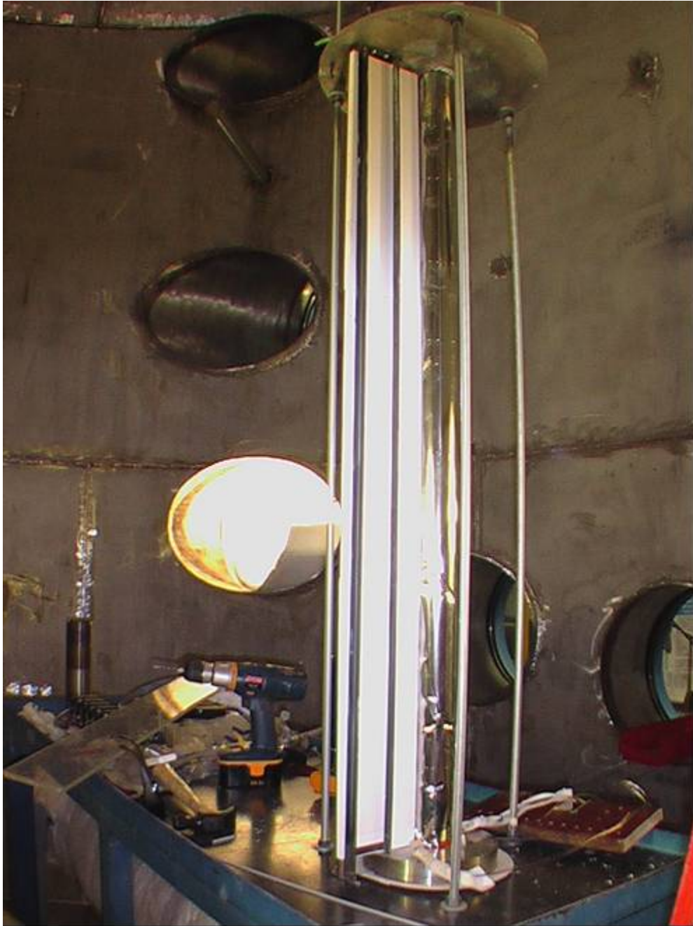
Figure 3.5 Stainless steel foil in place over quartz tube and ceramic positioning block is in place
