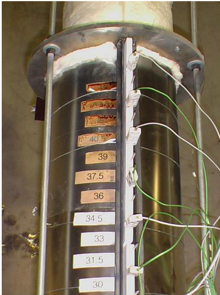
Figure 3.19 Outer insulation jacket after burn
