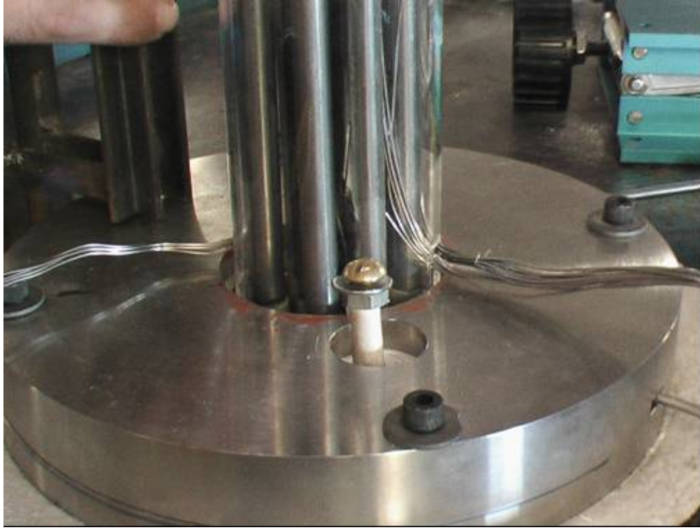
Figure 3.4 Quartz tube installed over heater bundle
