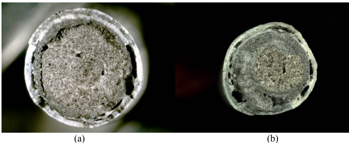
Figure 2.32 Photo image of burnt heater rod cross sections, (a) lower rod segment end detail, and (b) upper rod segment end detail
