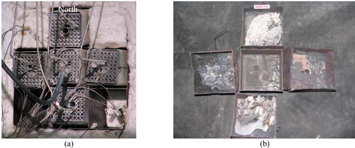
Figure 8.25 Post-ignition overhead photographs of (a) the apparatus and (b) the inlet air flow boxes
