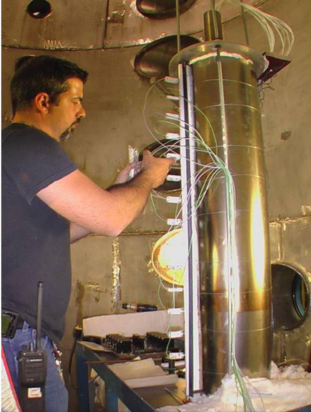
Figure 3.6 Installation of quartz wall TCs and light pipes into ceramic positioning block
