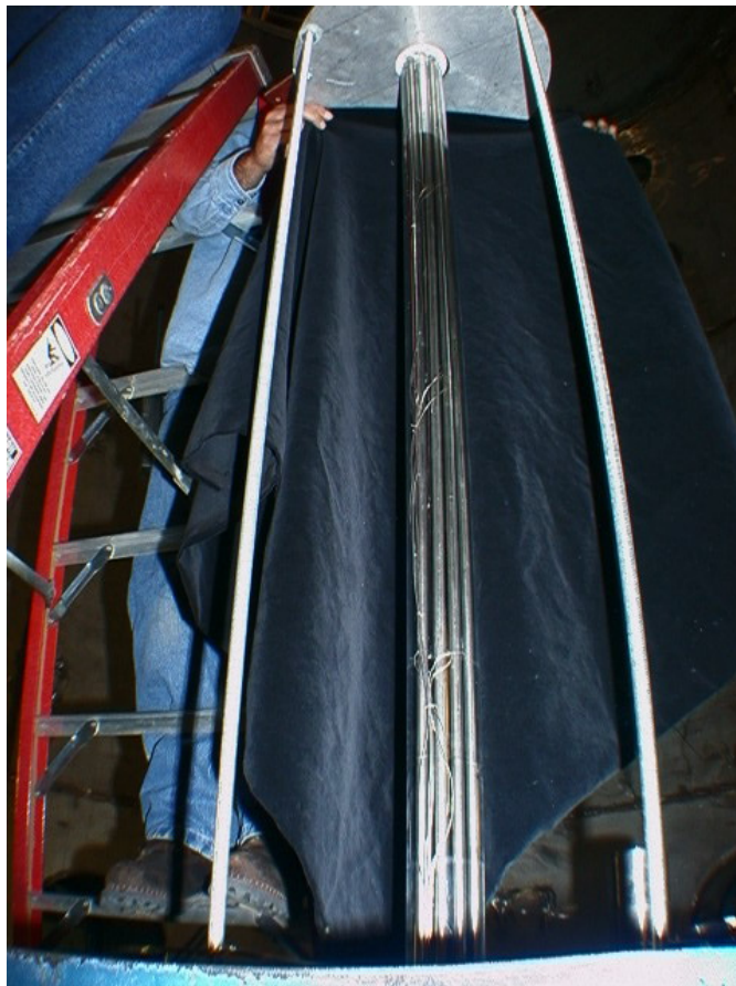
Figure 2.6 Quartz tube installed over heater bundle
