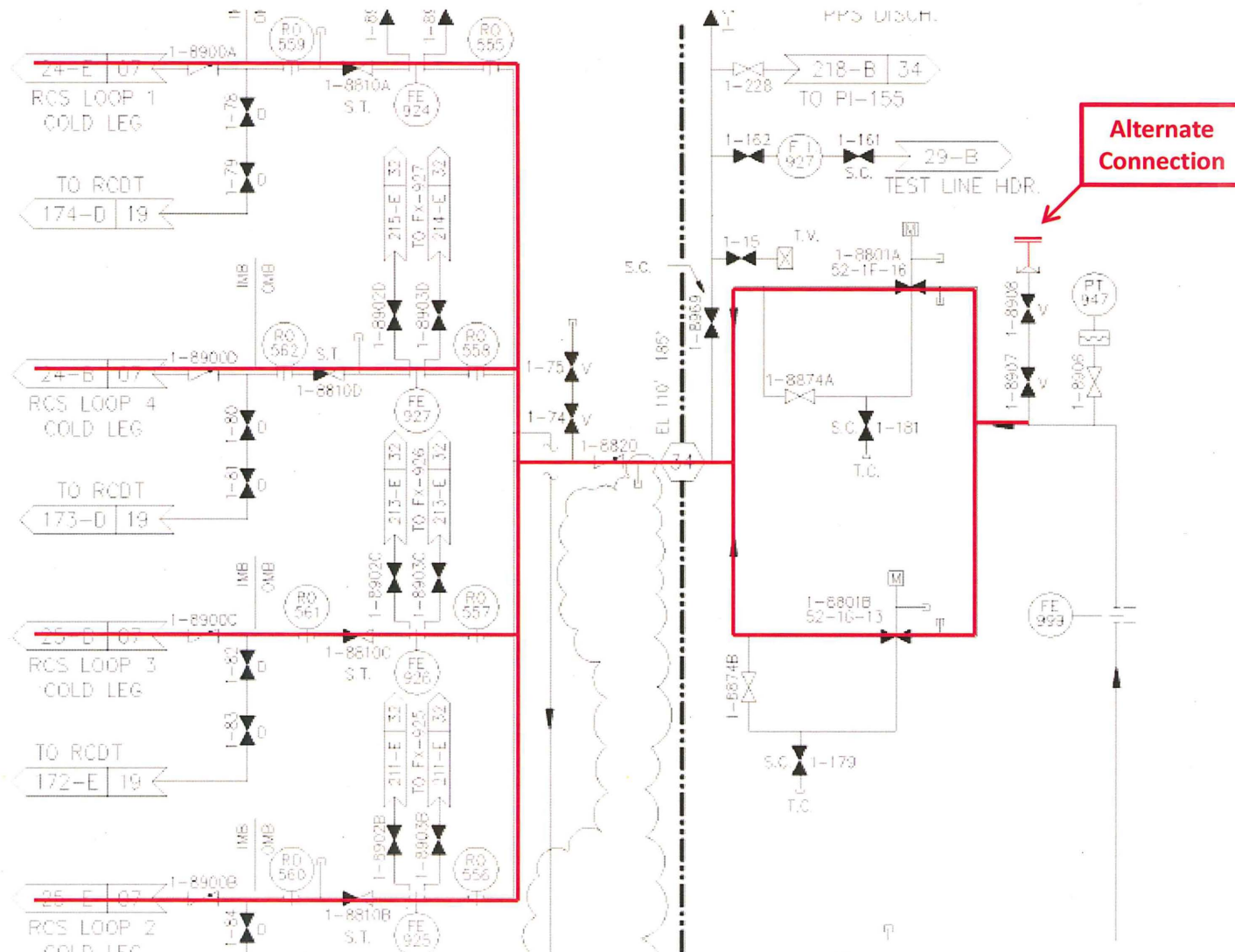
Figure 14 RCS Alternate Connection Point Unit 1
