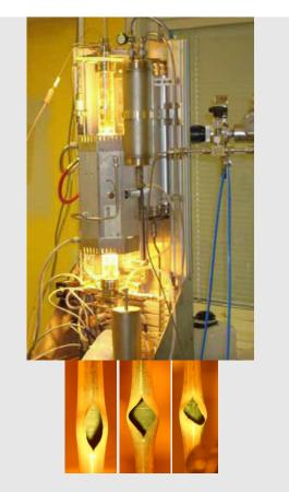
LOCA apparatus operating at 1,200 degrees Celsius at the Studsvik Nuclear AB laboratory (Sweden), where integral tests are being conducted on irradiated, high-burnup fuel rods. Rupture openings reveal the absence of fuel in the ballooned region caused by relocation and dispersal.
