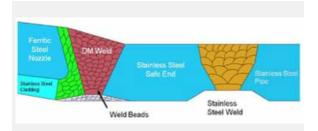
Cross-section of a dissimilar metal weld between a nozzle and safe end
