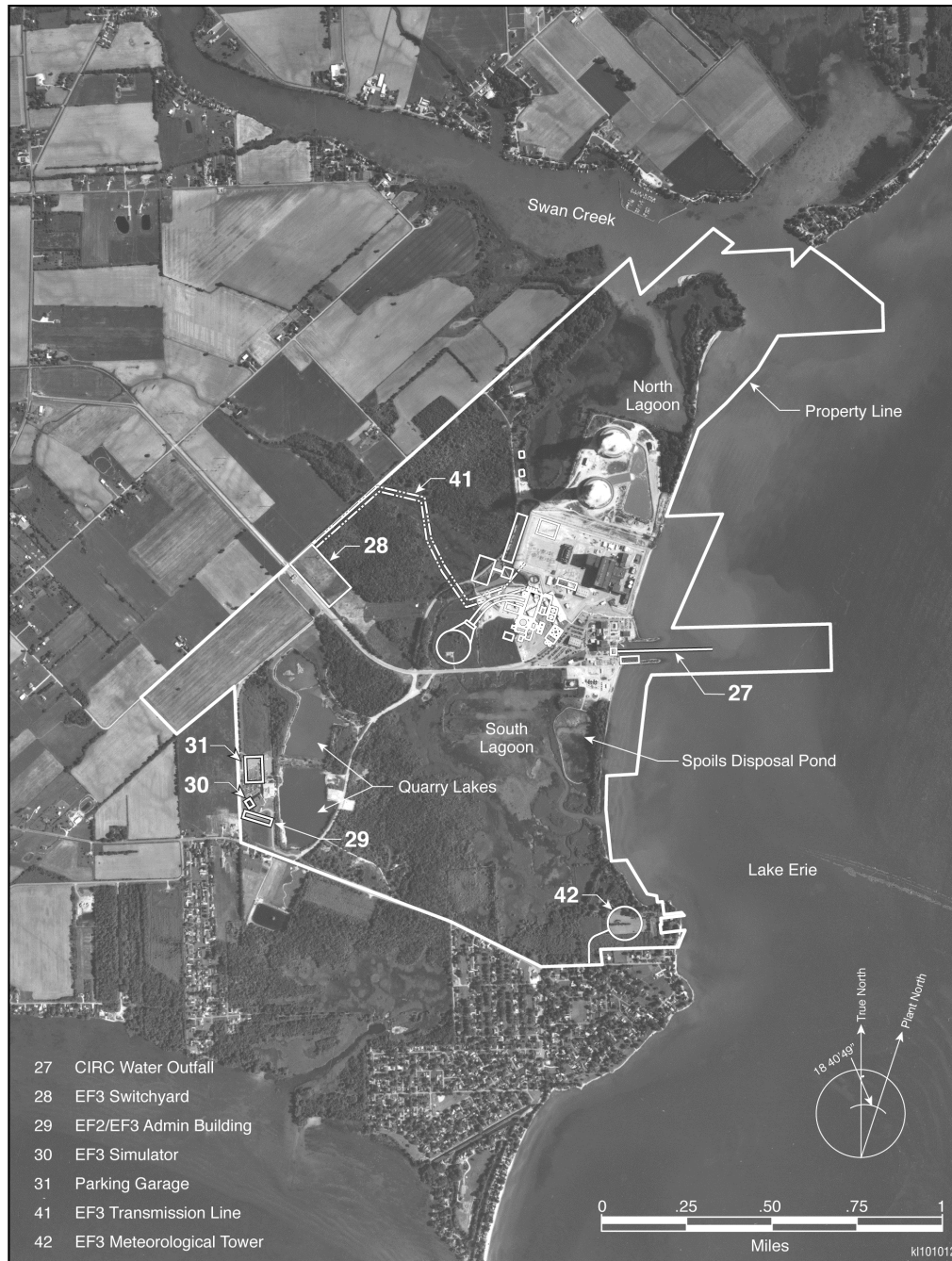
Figure 3-2. Fermi Site Layout Showing Existing and Proposed Facilities: Ancillary Facilities (Detroit Edison 2011b)
