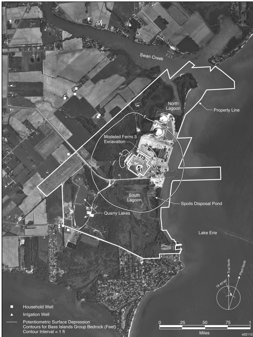
Figure 4-2. Modeled Drawdown of Groundwater in the Bass Islands Group as a Result of Dewatering for Fermi 3 Construction – Scenario 1 (Detroit Edison 2011a)
