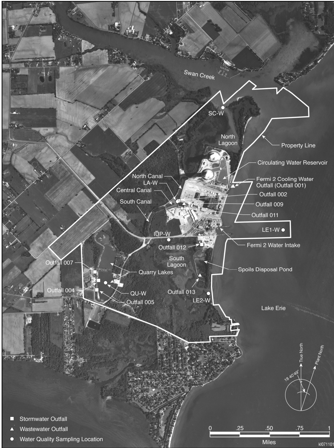
Figure 2-6. Surface Water Features, Discharge Outfalls, and Water Quality Sampling Locations on the Fermi Site
