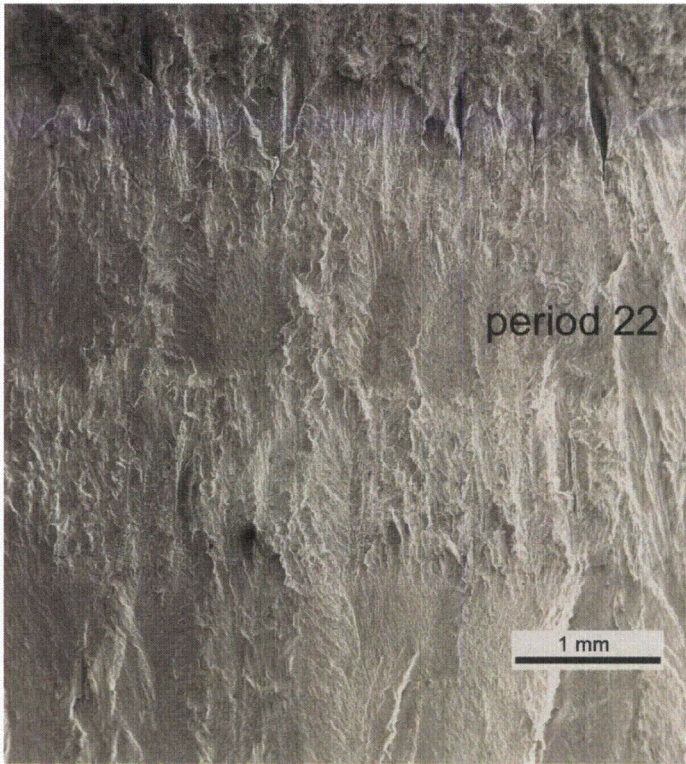
Figure 76. Fracture surface of specimen A152-TS-4 prior to period 22. Crack advance is from bottom to top.
