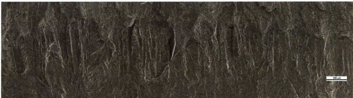
Figure 66. Intergranular cracking on the fracture surface of specimen A152-TS-2 between A and B in Fig. 65. Crack advance is from bottom to top.
