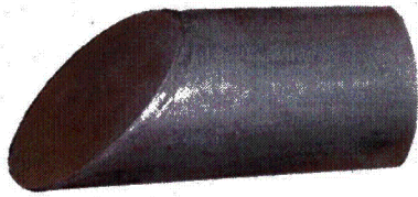
Figure 4.11a, Tangential Beam Port Insert
