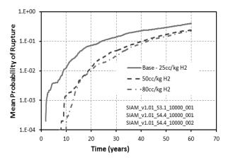
Figure 5-6 Effect of hydrogen on the mean probability of rupture<sup>3</sup>
