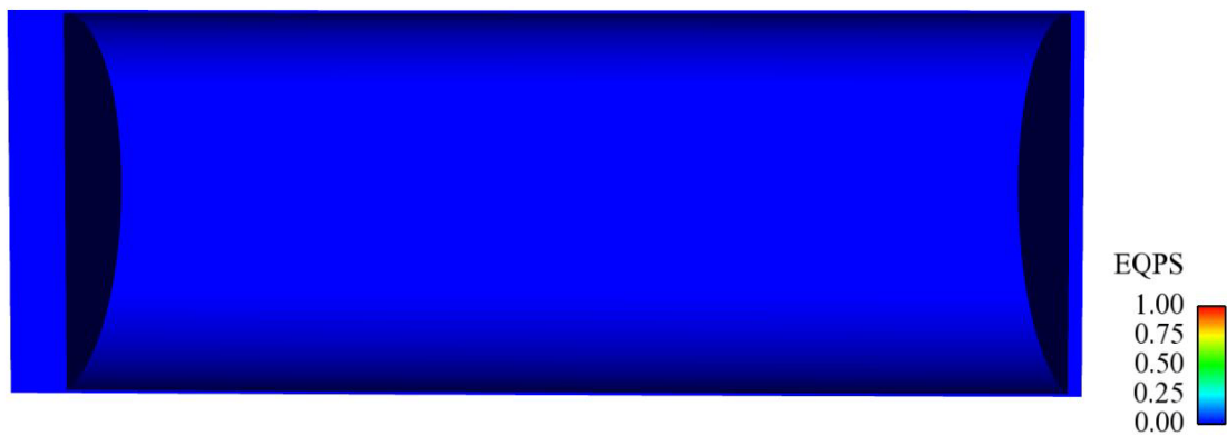
Figure C-20 Plastic strain in the interior welded canister of the Rail-Steel cask from the side impact at 48 kph (30 mph)
