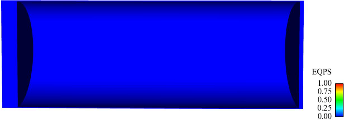
Figure C-21 Plastic strain in the interior welded canister of the Rail-Steel cask from the side impact at 97 kph (60 mph)
