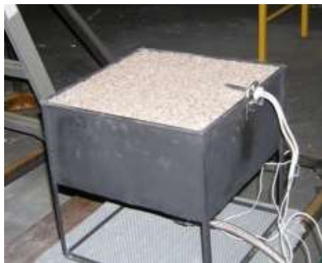
Figure 3-4 Photo of “sand box” diffusion burner
