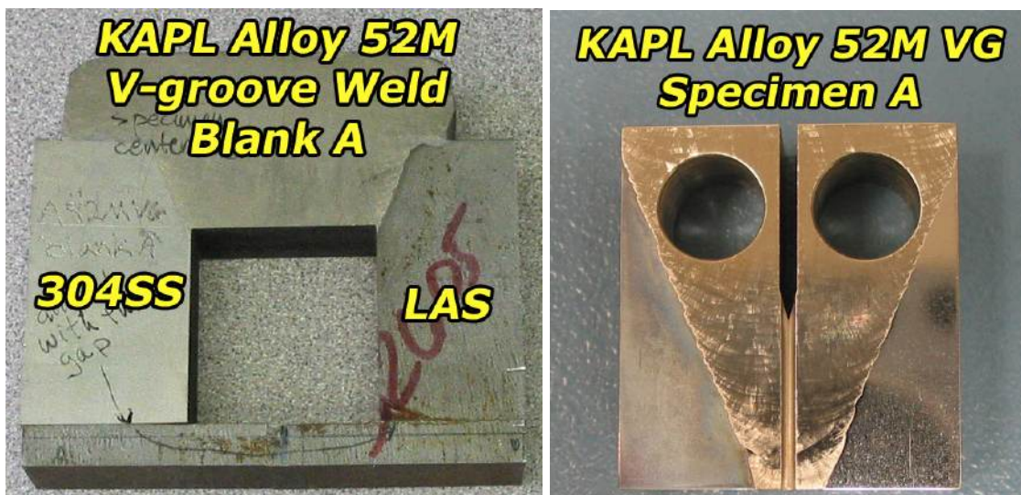
Figure 3.42 Photos of KAPL alloy 52M V-groove weld blank "A" and CT041 specimen machined from the blank.
