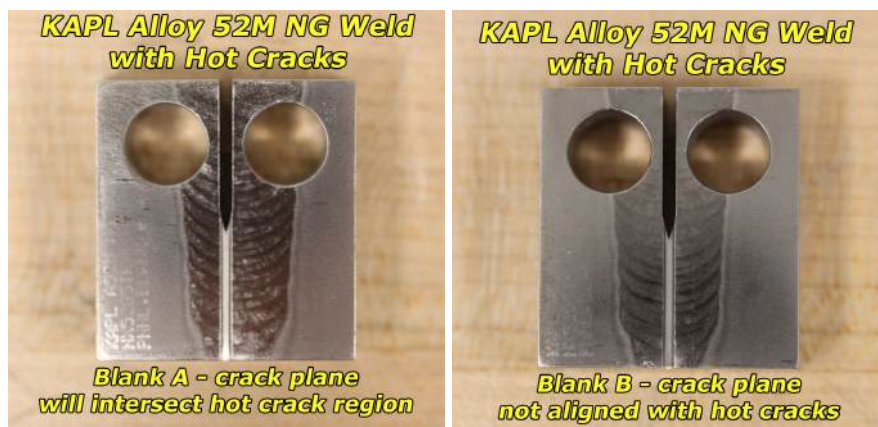
Figure 3.44 Photos of specimens cut from KAPL alloy 52M narrow gap weld containing hot cracks. Blank A (CT042) is positioned off-center and near the bottom of the weldment to intersect a high density of weld cracks, while blank B (CT043) is positioned near the center of the weld where no weld cracks were observed.
