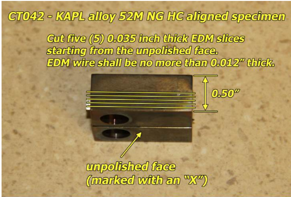
Figure 3.60 Post-test serial sectioning plan for KAPL alloy 52M NG weld specimens with hot cracks (CT042 & CT043).
