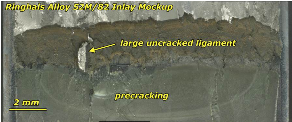
Figure 3.91 Crack growth surface of Ringhals alloy 52M/82 specimen CT030.
