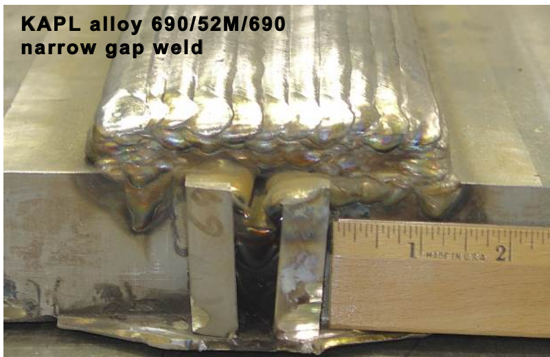
Figure 3.40 Alloy 52M welds from KAPL: (a) dissimilar metal V-groove weld of alloy EN52M joining 304 SS and carbon steel and (b) alloy EN52M narrow gap weld joining alloy 690. The thin rectangular bars at the front of the weld are run-off tabs to help start the weld. The weld itself is between the two large plates. Additional weldment was placed on top of the mockups to create sufficient size to cut CT specimens.
