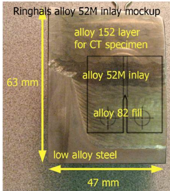
Figure 3.82 Profile of Ringhals alloy 52M inlay mockup weld received from Westinghouse. Alloy 52M inlay is 10 mm thick.
