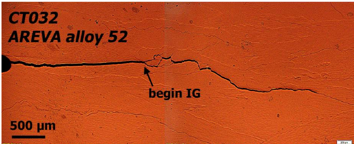
Figure 3.38 Side surface optical image of cracking in the AREVA alloy 52 specimen (CT032) showing both TG and IG growth.
