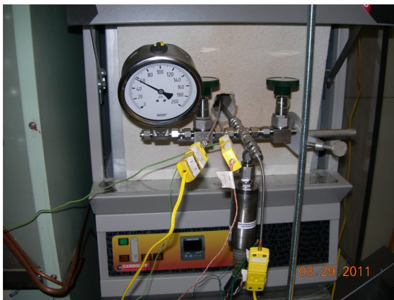
Figure 3-21. A photograph showing the pressure gauge used to check the pressure transducer performance.
