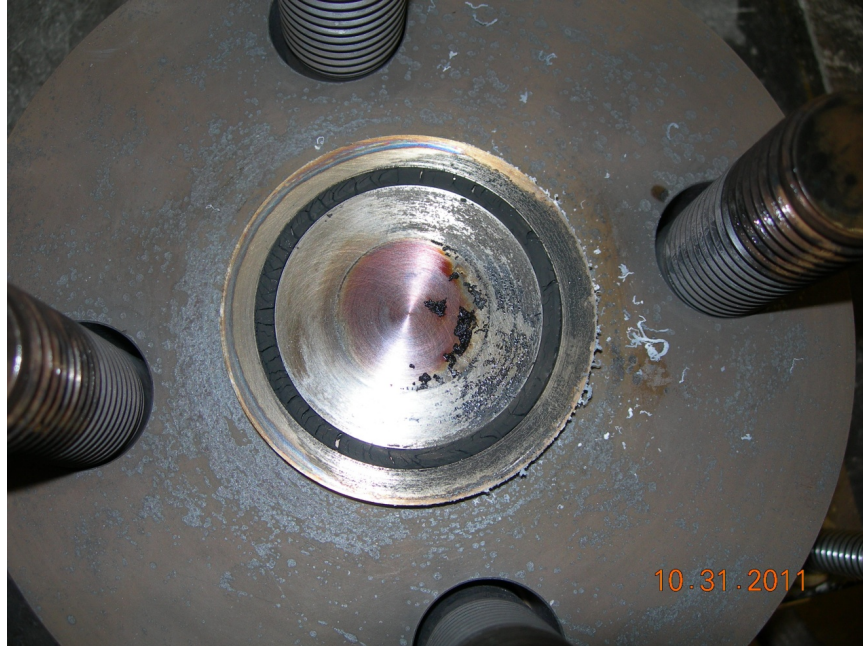
Figure 3-39. Photograph of the ethylene-propylene compound O-ring after thermal exposure.
