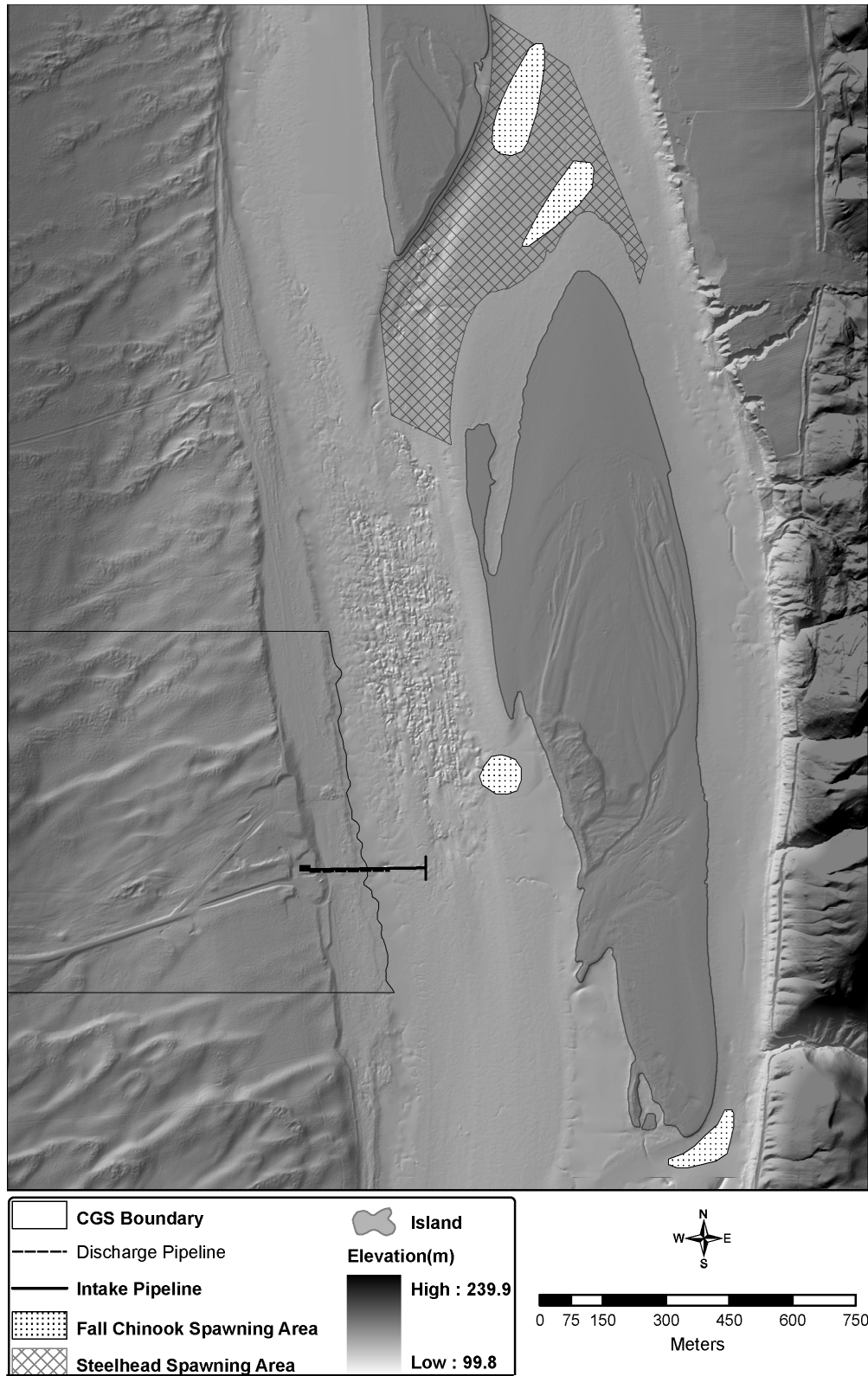
Figure 2.1-5. Location of pumphouse, pipelines, intakes, and outfalls
