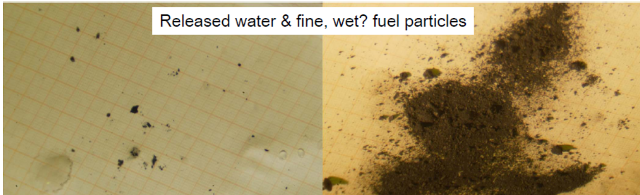
Figure 4-30 Fuel residue from posttest disassembly of IFA-650.9 (Ref. 46)
