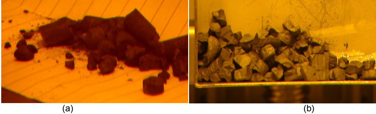
Figure 4-42 Images of fuel particles collected from test rod (a) 196 and (b) 198 revealing large fragments
