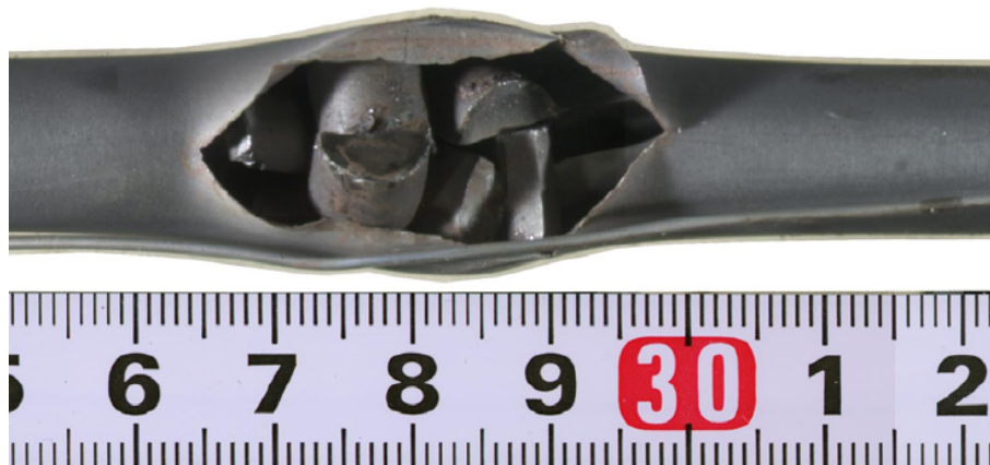
Figure 4-26 Ballooned region with relocated fuel in the Halden IFA-650.2 test (Ref. 61)
