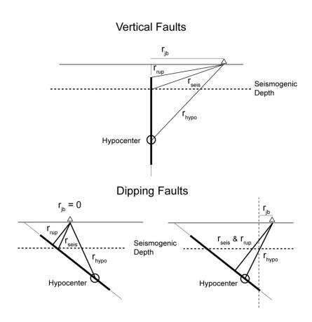
Figure B-4. Distance Metrics for the Location of a Site with Respect to the Source of an Earthquake (Abrahamson and Shedlock, 1997).
