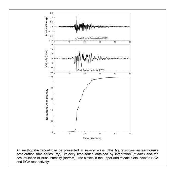
Figure B-5. An Earthquake Acceleration Time Series, and Velocity Time Series, and the Accumulation of Arias
