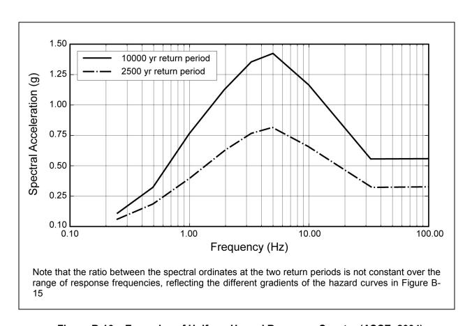
Figure B-16. Examples of Uniform Hazard Response Spectra (ASCE, 2004).
