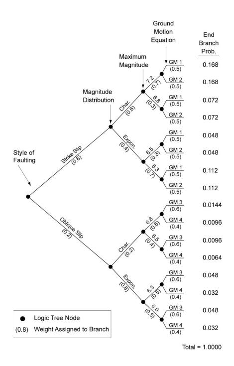
Figure B-22. Logic-Tree for a Single Fault Source (McGuire, 2004).
