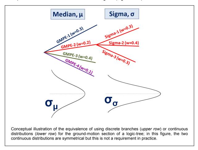
Figure B-24. Conceptual Illustration of the Equivalence of Using Discrete Branches or Continuous Distributions for the Ground-Motion Section of a Logic-Tree.
