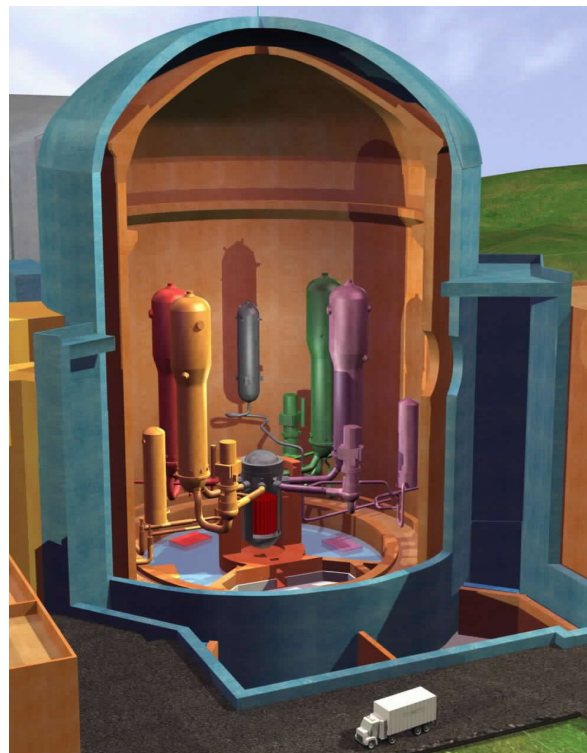
The U.S. EPR containment building (Courtesy: AREVA NP)
