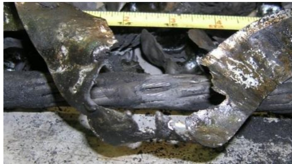
Figure 7.47: Removal of the zinc wrap and charred insulation material reveal the bare copper conductors.
