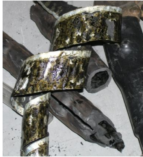
Figure 7.36: Oily residue found between the jacketing material and zinc wrap.
