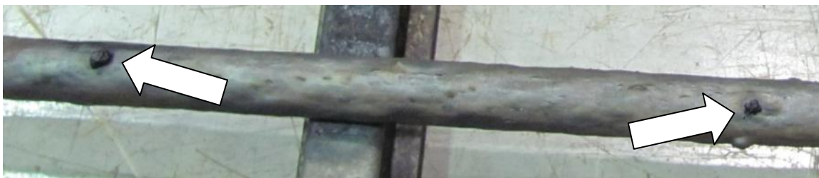
Figure 7.20: Dried liquid coming through the jacket material during post-test examination.
