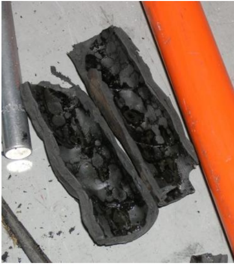
Figure 7.36: Oily residue found between the jacketing material and zinc wrap.
