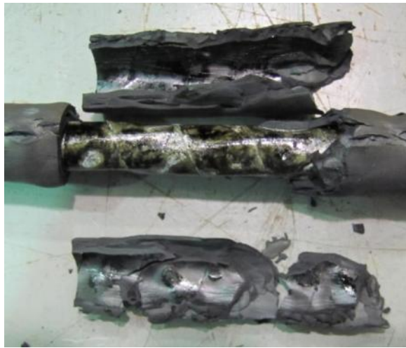
Figure 7.13: Oily residue found between the jacket and zinc wrap of Item D.
