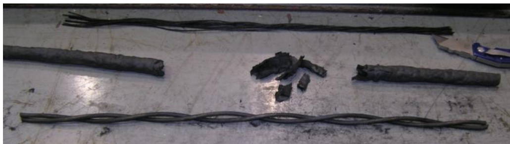
Figure 7.6: Conductors from the section of Item B located in the center of Penlight.
