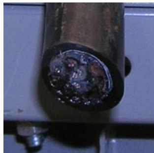
Figure 7.40: Liquid observed from cut end of thermal response cable during Test K4.
