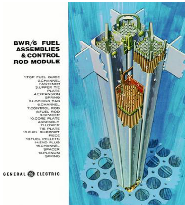
Figure 3 BWR Fuel Assembly [ http://www.nucleartourist.com/images/bwrfuel1.jpg ].
