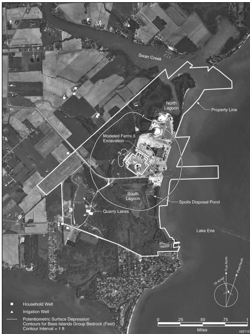
1 2 Figure 4-2. Modeled Drawdown of Groundwater in the Bass Islands Group as a Result of 3 Dewatering for Fermi 3 Construction – Scenario 1 (Detroit Edison 2011a)
