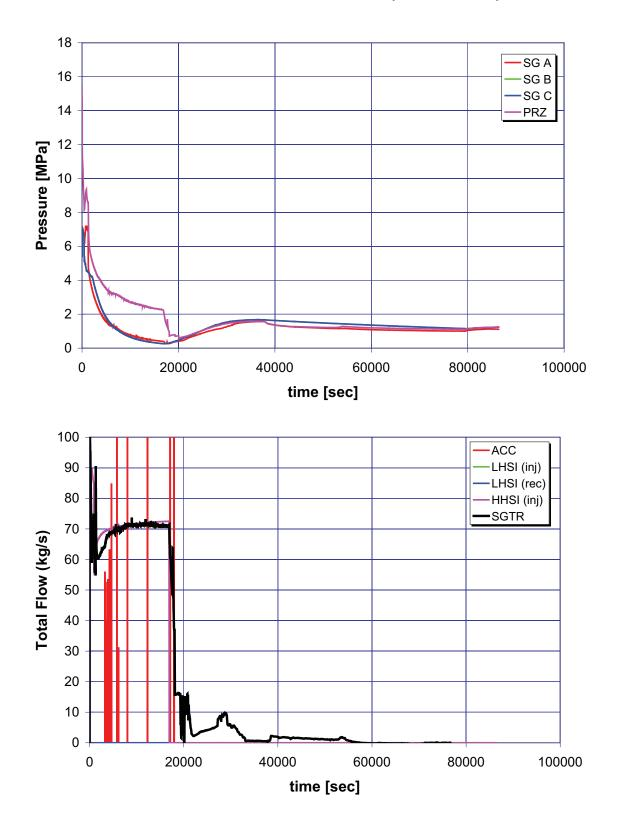
A.4.5 Case 5: Five Tubes, Secure One HHSI Pump, and Stuck-Open SG PORV
