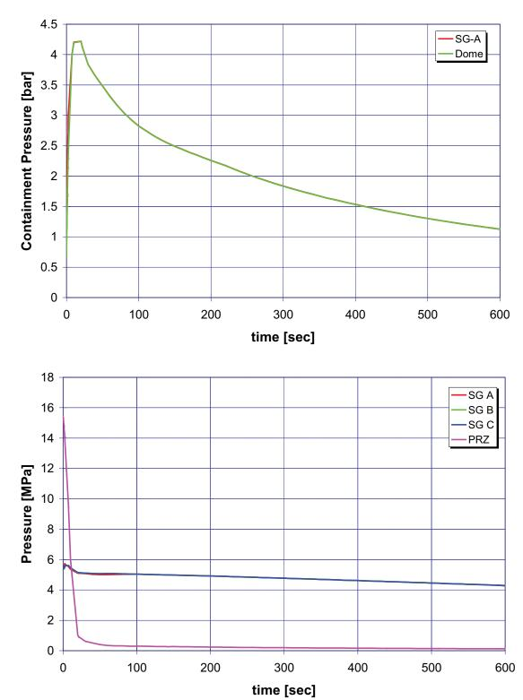
A.6.10 Case 10: Double-Ended Cold-Leg Break LOCA, No HHSI, One LHSI, and No ACC
