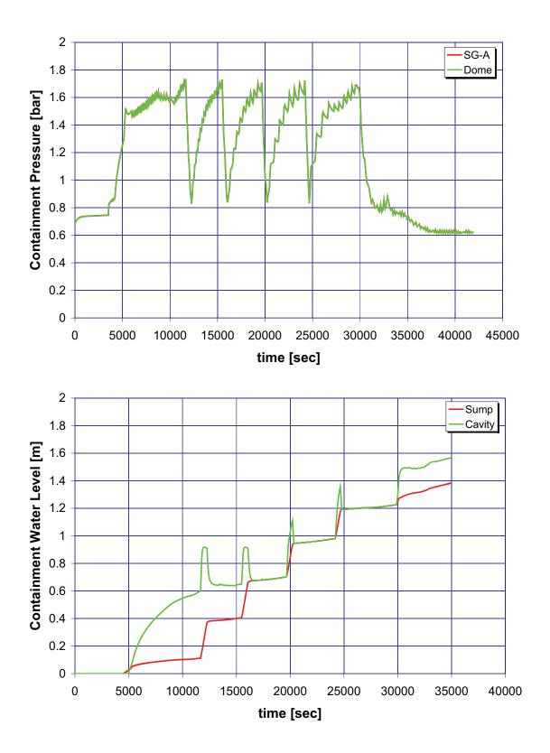
A.3.3 Case 3: 113.9-Percent Power Level, Reactor Trip on Low-Low SG Level
