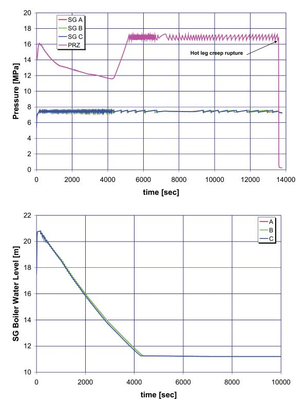
A.5.3 Case 3: Station Blackout without Turbine-Driven Auxiliary Feedwater (21 gpm)
