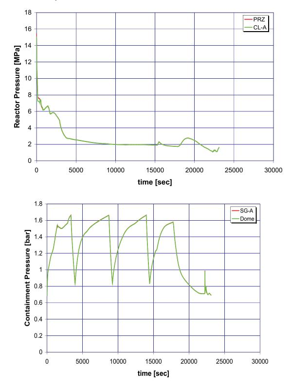
A.6.29 Case 29: 2-Inch Break LOCA, One HHSI, One LHSI, and No ACC, without Auxiliary Feedwater
