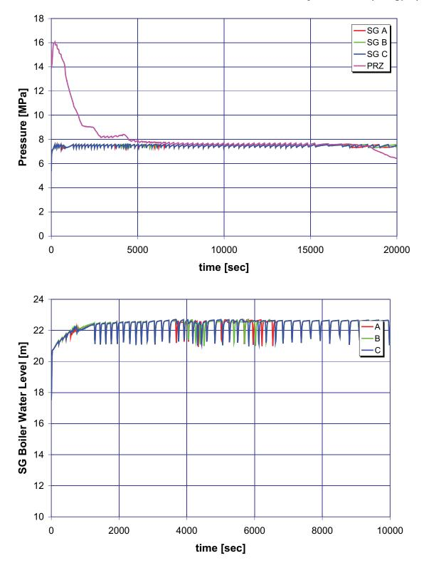
A.5.8 Case 8: Station Blackout with Turbine-Driven Auxiliary Feedwater (182 gpm)
