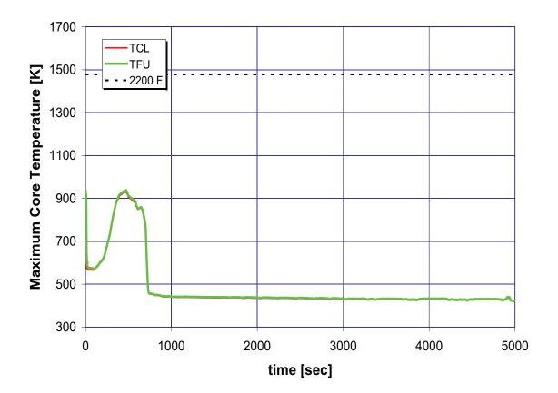
A.6.27 Case 27: 2-Inch Break LOCA, One HHSI, No LHSI, and One ACC, without Auxiliary Feedwater
