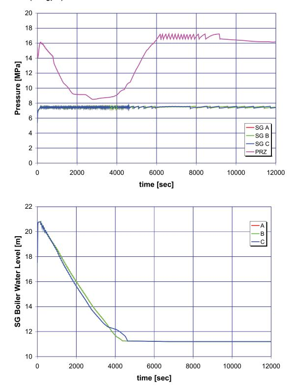
A.5.7 Case 7: Station Blackout without Turbine-Driven Auxiliary Feedwater (182 gpm)
