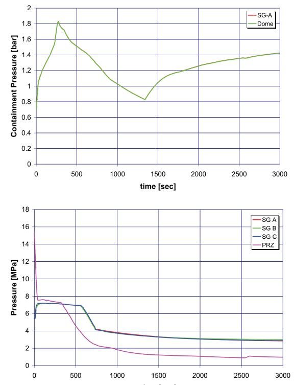
A.6.28 Case 28: 4-Inch Break LOCA, One HHSI, No LHSI, and One ACC, without Auxiliary Feedwater
