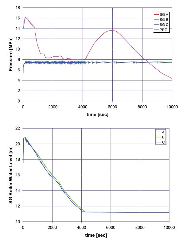
A.5.1 Case 1: Station Blackout without Turbine-Driven Auxiliary Feedwater (500 gpm)
