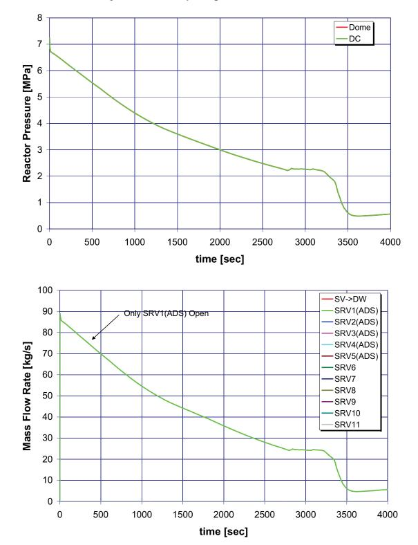
B.1.3 Case 3: Safety Relief Valve Opening and CRD 2 at 10 Minutes
