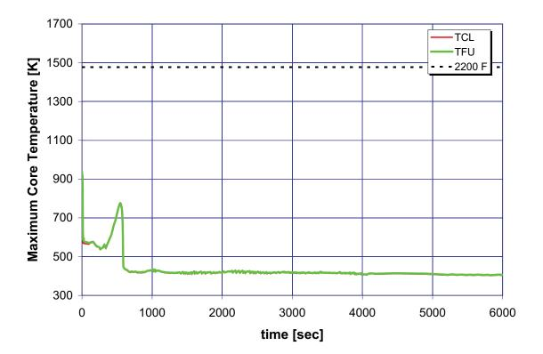
A.6.17 Case 17: 6-Inch Break LOCA, One HHSI, No LHSI, and One ACC, without Auxiliary Feedwater
