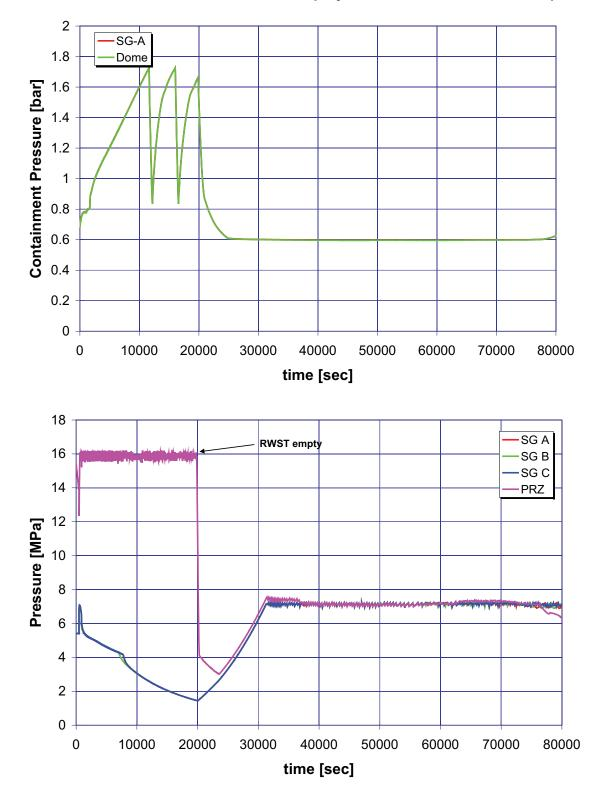
A.2.8 Case 8: 0.5-Inch Break LOCA with Sprays and PRZ PORV Not Stuck Open
