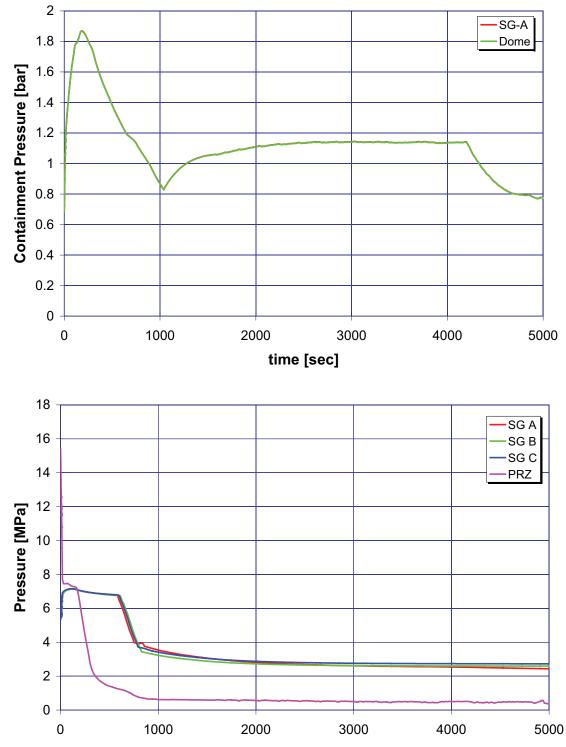
A.6.26 Case 26: 6-Inch Break LOCA, No HHSI, One LHSI, and One ACC, without Auxiliary Feedwater
