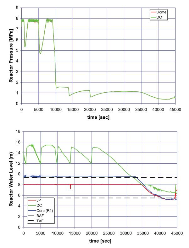
B.2.10 Case 10: Station Blackout and HPCI and SRV Stuck Open
