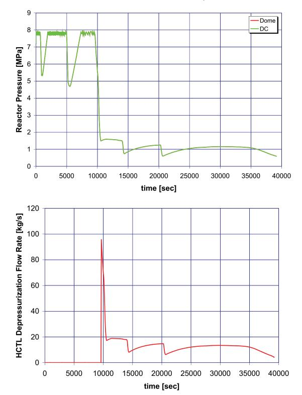
B.2.8 Case 8: Station Blackout and HPCI and HCTL Depressurization
