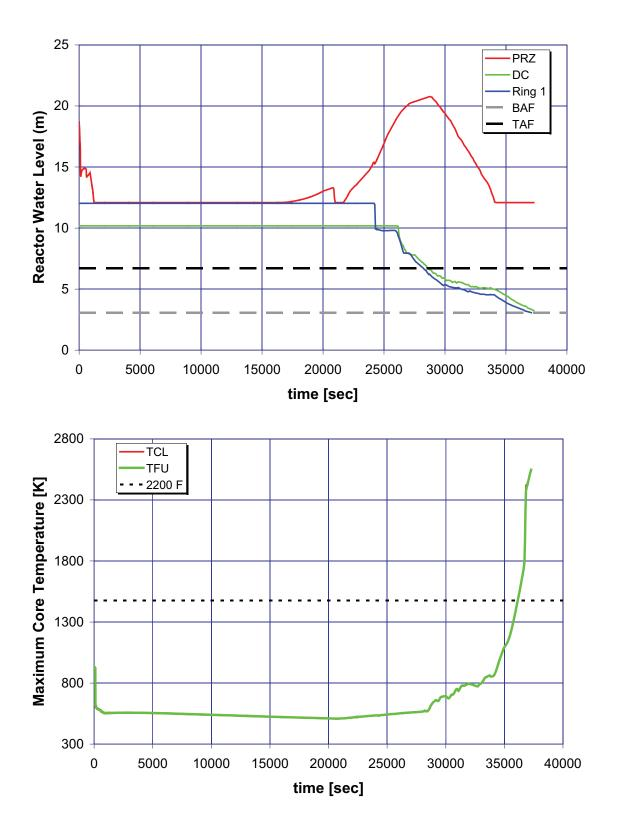
A.2.2.2 Case 2b: 1-Inch Break LOCA with Sprays, Secure HHSI Pumps, and Secondary Cooldown
