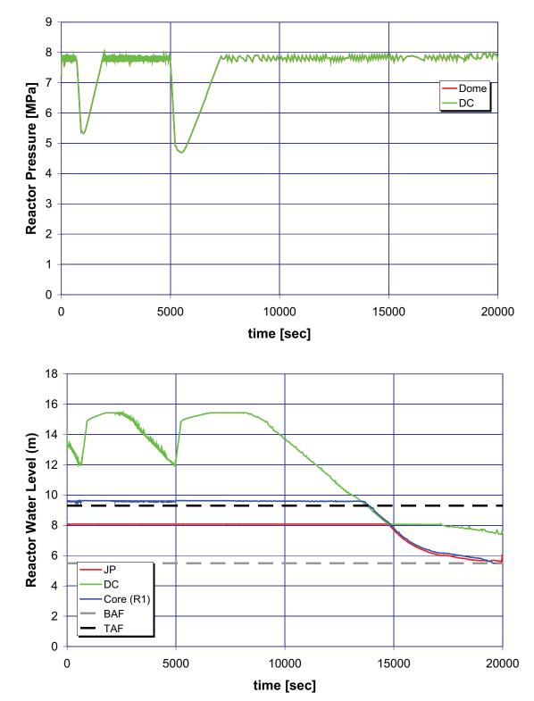
B.2.9 Case 9: Station Blackout and HPCI and 2-Hour Direct Current
