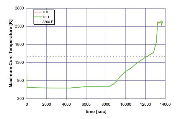
A.5.4 Case 4: Station Blackout with Turbine-Driven Auxiliary Feedwater (21 gpm)
