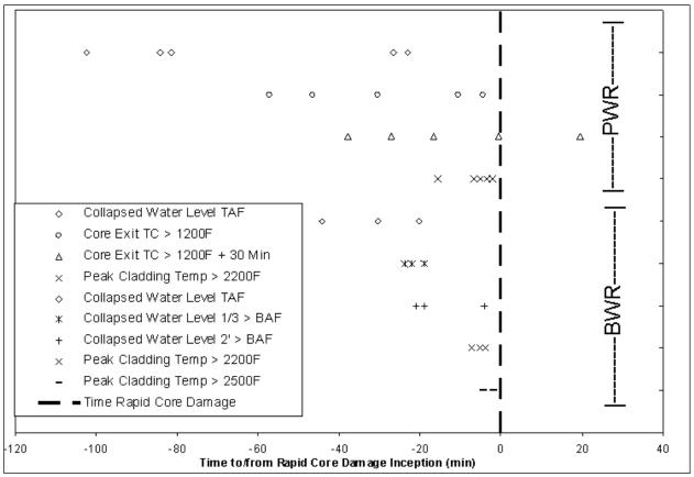
Figure 1 Summary of Core Damage Surrogate Calculations (1,200 °F = 649 °C; 2,200 °F = 1,204 °C; 2,500 °F = 1,371 °C)
