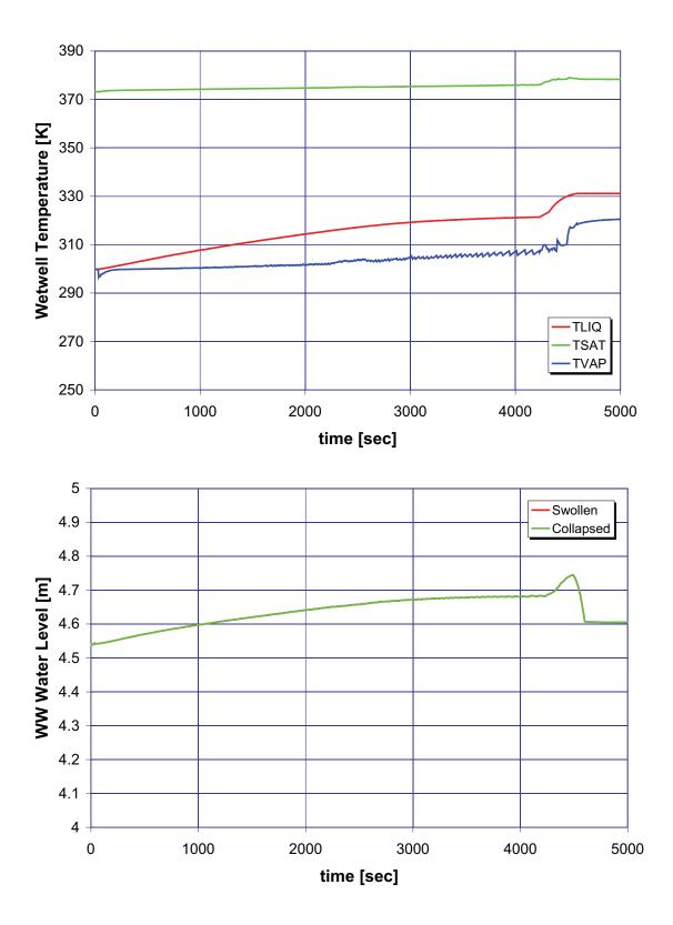
B.2.2 Case 2: Station Blackout and Safety Relief Valve Open at t = 0
