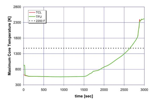
A.6.16 Case 16: 6-Inch Break LOCA, One HHSI, One LHSI, and No ACC, without Auxiliary Feedwater
