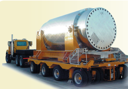
Empty storage transport container on a semi tractor-trailer rig.
