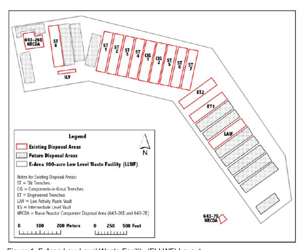
Figure 1. E-Area Low-Level Waste Facility (ELLWF) Layout
