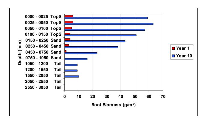
Figure 1. EDYS simulations of root development on the water-balance cover over tailings at the Mineral Hill TVX mine site, Montana.
