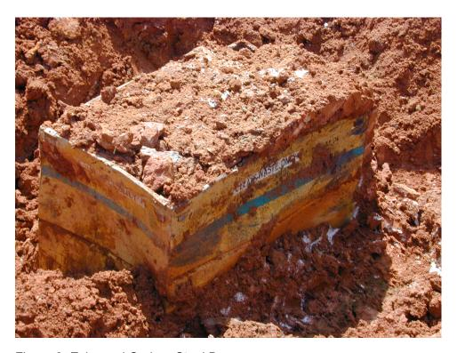
Figure 3. Exhumed Carbon Steel Box
