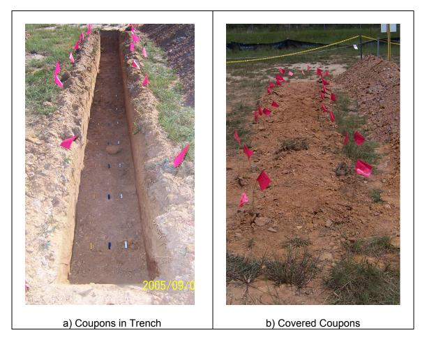
Figure 4. Corrosion Coupon Monitoring Trench
