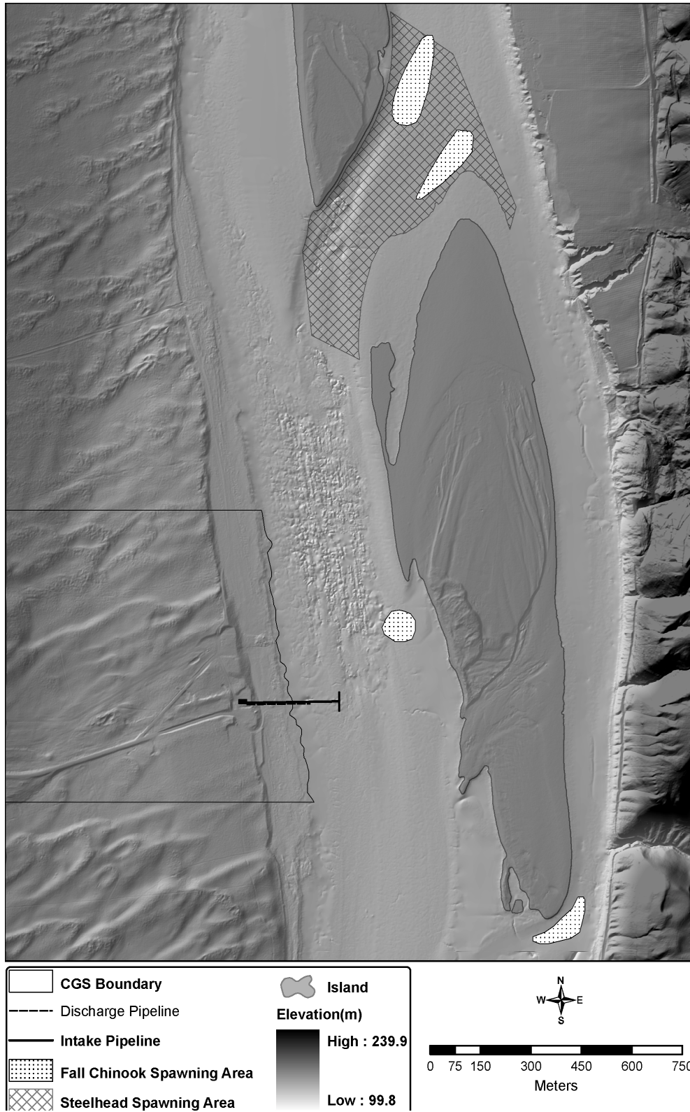
Figure D-1-5. Location of pumphouse, pipelines, intakes, and outfalls showing historical steelhead and fall Chinook salmon spawning locations
