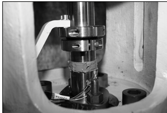
Figure 6: View of Instrumented Stem with Position Indication Arm
