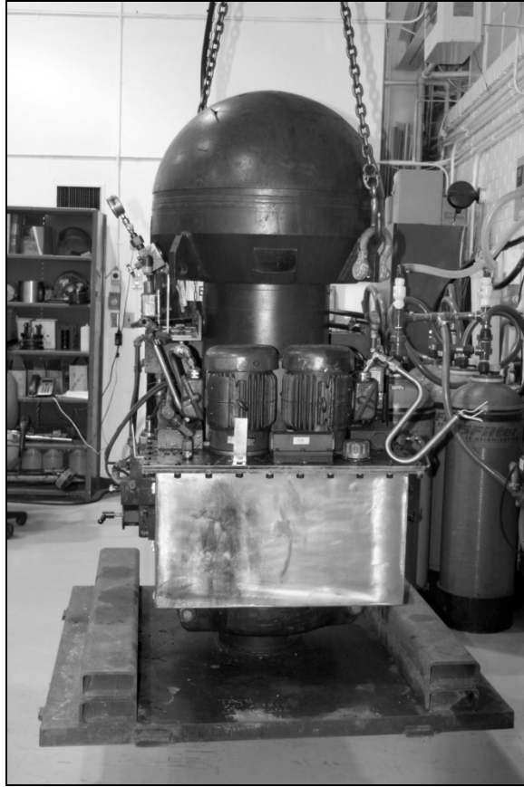
Figure 6, Flowserve Edward Type A, Gas / Hydraulic Actuator After the Design Basis Accident (DBA) Tests.
