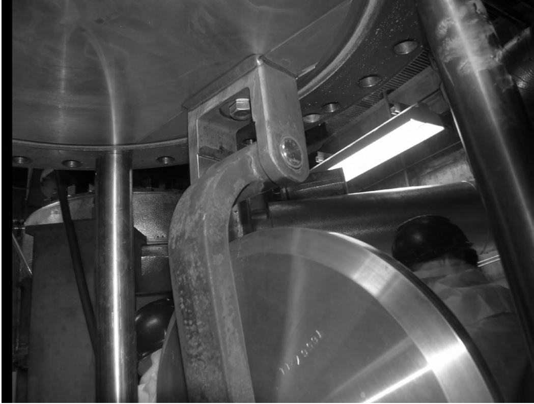
Figure 4 – Valve Bonnet Hung Assembly Upper
