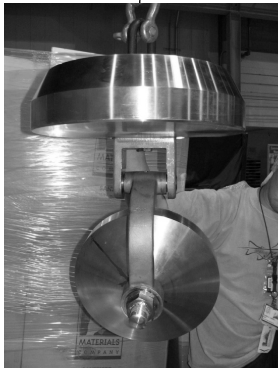
Figure 4: Depiction of the top of the disk getting caught under the top of the seat and a photograph of the bonnet hung disk assembly
