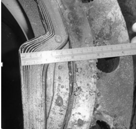
Figure 3 Radial Buckling of a Sprial Wound Gasket
