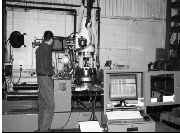
Figure 7: Picture of Production Functional Testing of an MOV with Full Instrumentation and Test Data Collection.
