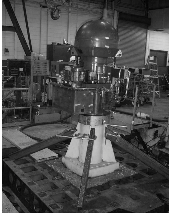
Figure 4, Flowserve Edward Type A, Gas / Hydraulic Actuator During the Dynamic Seismic Tests, Triaxial – Random Multi-Frequency Input.
