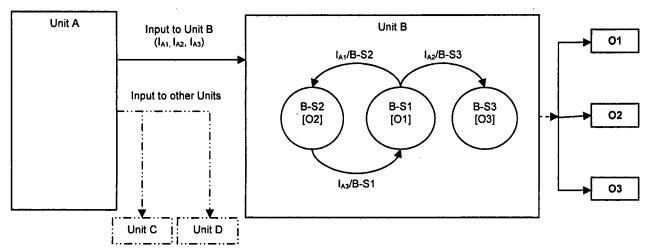
Figure 2: Unpredictable fault propagation in software
