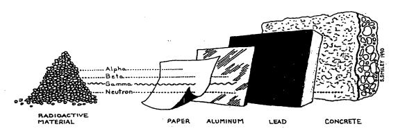
Figure 3: As radiation travels, it collides and interacts with other atoms and loses energy. Alpha particles can be stopped by a sheet of paper, and beta particles by a thin sheet of aluminum. Gamma radiation is shielded by highly dense materials such as lead, while hydrogenous materials (those containing hydrogen atoms), such as water and concrete, are used to stop neutrons.
