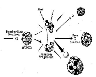
Figure 5: When a heavy atom, such as uranium-235 is split or fissioned, heat, free neutrons, and fission fragments result. The free neutrons can then strike neighboring atoms causing them to fission also. In the proper environment, this process can continue indefinitely in a chain reaction.
