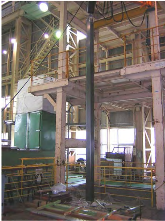
Figure 3-33 Mockup of A BWR Fuel Assembly
