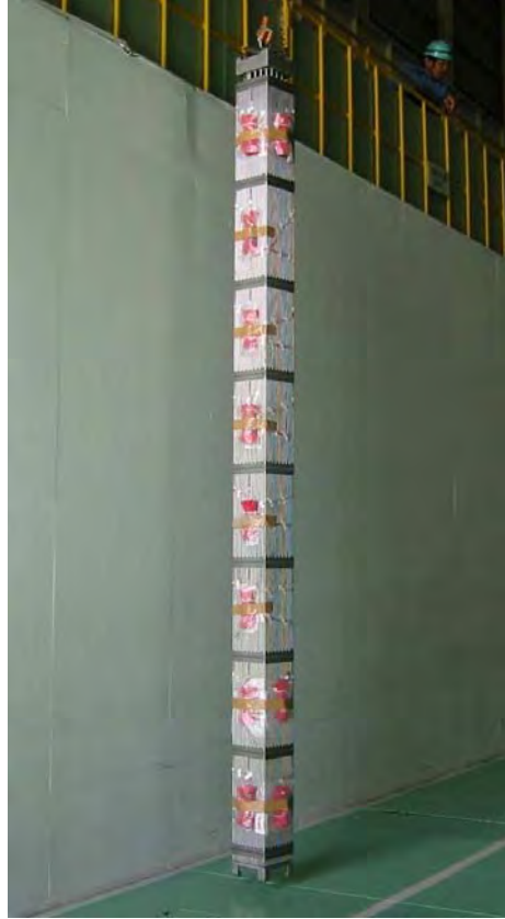
Figure 3-20 Mockup of A PWR Fuel Assembly
