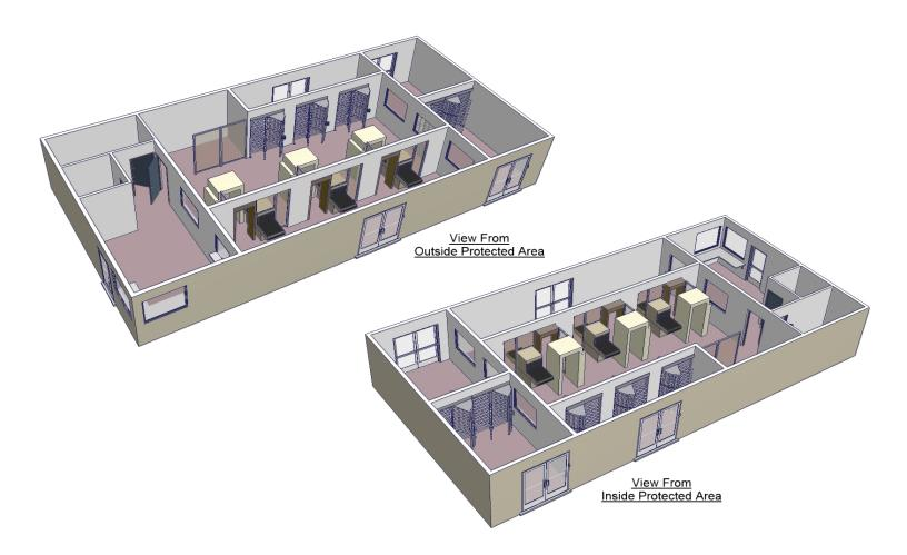
Figure 19: The protected area personnel access control portal viewed from outside and inside the protected area
