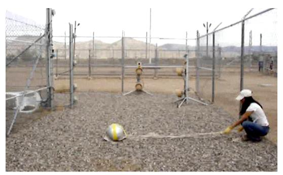
Figure 9: Testing microwave sensors with an aluminum sphere.
