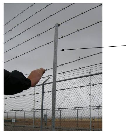
Figure 30: A hanging yardstick allows for easy measurement of the deflection possible on a taut wire sensor before an alarm occurs.
