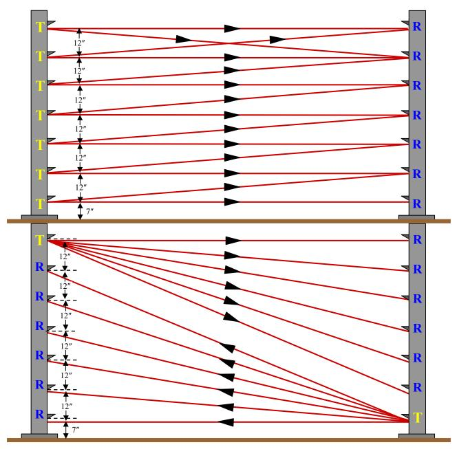
Figure 24 below provides examples of the available designs of active infrared systems with varying transmitter, receiver and beam configurations.
