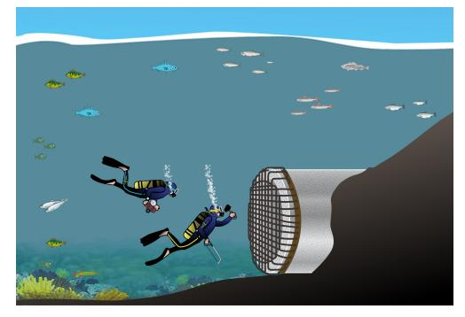
Figure 57: An example of a fiber-optic grid covering a water intake channel.
