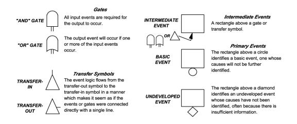
Figure 84: Symbols used in the graphical representation of a fault tree.
