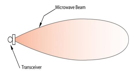
Figure 39: A common interior microwave antenna propagation pattern.
