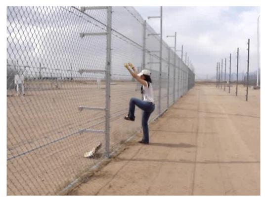
Figure 35: Test climbing the fence from the outer (unprotected) side.
