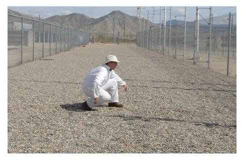
Figure 22: The "duck walk" seems to produce the smallest disturbance in a ported coaxial system and is therefore ideal to use to test the system.
