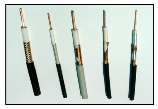
Figure 18: Examples of ported coax cables.
