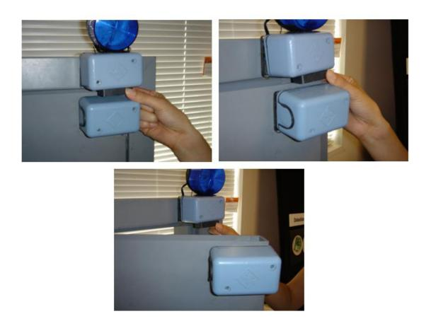
Figure 38: Demonstration of introducing an external magnetic field to a BMS. Note that this procedure is much more difficult to accomplish than the photos would suggest.
