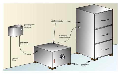
Figure 51: Example of a capacitance sensor installation.
