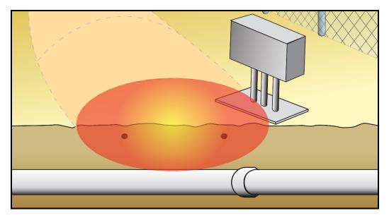
Figure 21: Metal objects or utilities located within the detection volume of a ported coax system may create areas of poor detection.
