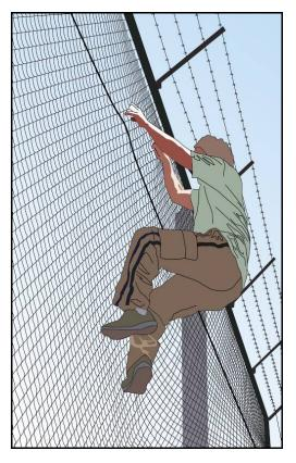
Figure 31: This diagram illustrates the deflection caused by climbing on chain-link fence fabric; this disturbance of the fabric is one of the ways that fence disturbance sensors work.
