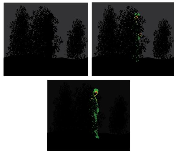
Figure 81 These drawings illustrate the use of an enhanced night vision device, or fusion technology. The top left drawing shows such a device set for 100 percent  $l^2$  (Image Intensification) use. The top right drawing shows it set for about 50 percent  $l^2$  and 50 percent infrared use. The bottom drawing shows it set for 100 percent infrared use. Obviously, different situations would require different settings to gain optimal information.
