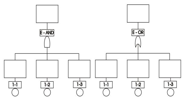
Figure 83: Fault trees allow analysts to map events and their potential causes. (Refer to the next figure for explanations of symbols.)
