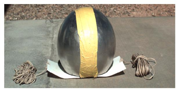
Figure 8: An aluminum sphere is commonly used for testing the potential success of a crawler against a microwave detection system.
