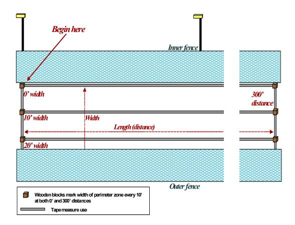
Figure 78: Preparation for measuring perimeter lighting illumination.
