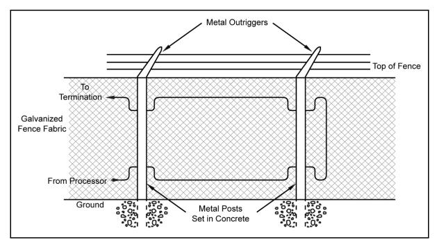
Figure 32: Typical installation of strain-sensitive cable.
