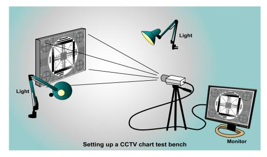
Figure 62: Example of a resolution chart test setup.
