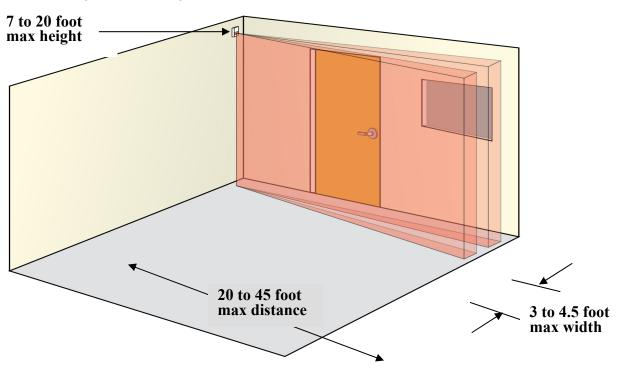
Figure 46: An example of a curtain PIR application.
