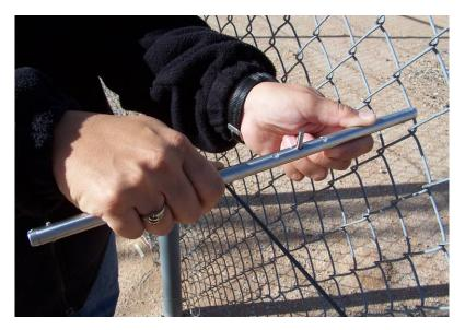
Figure 34: An example of a fence-cut simulation tool in use.
