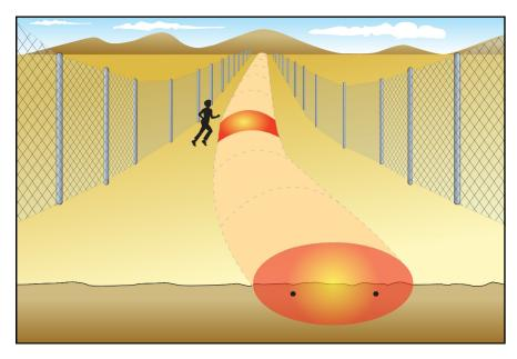
Figure 16: An illustration of the covert zone of detection for a ported coax sensor.
