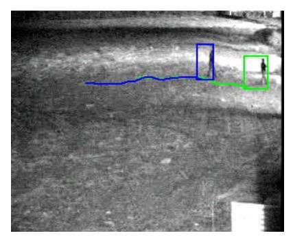
Figure 69: Video motion detection image showing intruder tracking.
