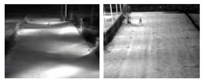
Figure 74: The scene at left has a high light-to-dark ratio of approximately 20:1, which is not considered sufficient. The scene at right has a low light-to-dark ratio of approximately 4:1, which maximizes the ability to assess an alarm.
