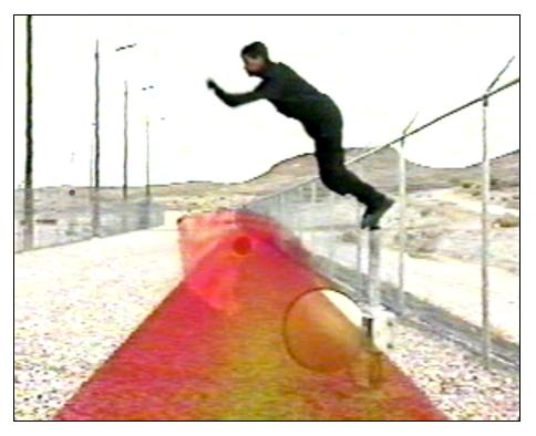
Figure 6: This scene taken from a test of microwave sensors shows the possibility of an attacker using the microwave structure as an aid to jump over its own detection zone. Note: The microwave patterns shown in the photo were added for illustration purposes.
