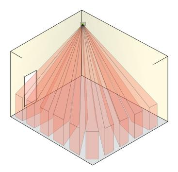
Figure 45: A PIR sensor's detection pattern is subdivided into solid angular segments; a specific number of segments must detect an anomaly before the sensor will signal an alarm condition.
