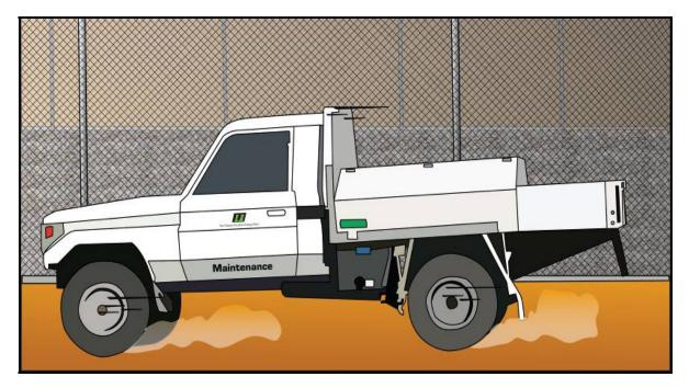
Figure 19: Sources of nuisance alarms for ported coaxial cable detection systems include nearby moving vehicles, larger animals, large and wet plants moving in the wind, and moving water, as well as the ripples caused by wind blowing across standing water.
