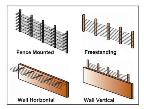
Figure 12: Various configurations for electric field sensors.
