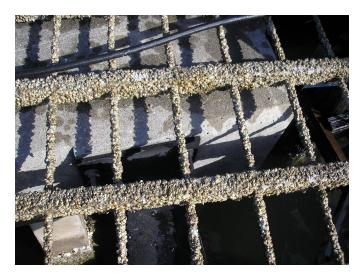
*Figure 58:* This fiber-optic grid was tested under water for about 6 weeks and shows biofouling through barnacles, which can eventually degrade the integrity of the materials.
