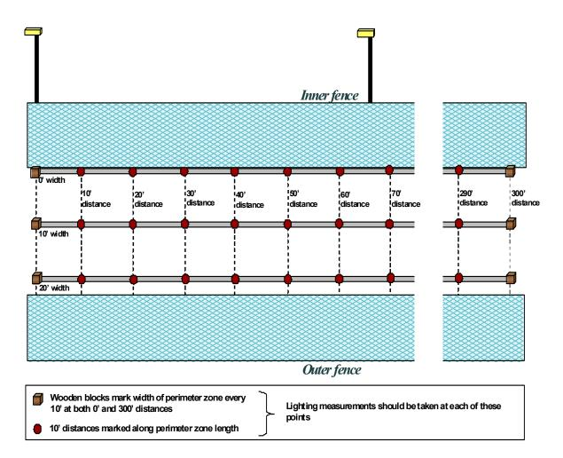
Figure 79: Points at which to measure light readings.
