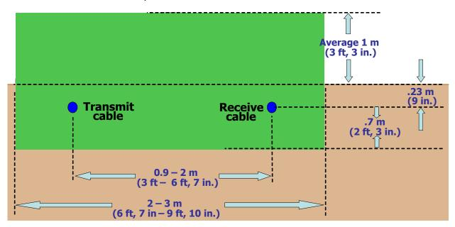
Figure 17: A typical installation and detection envelope (green oval) for a ported coax sensor.
