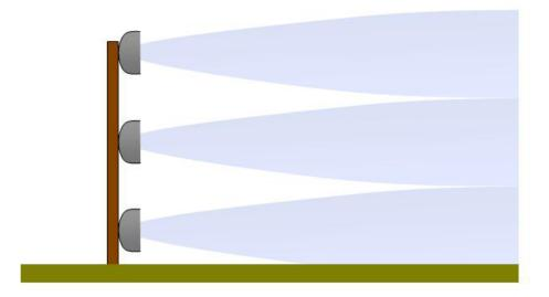
Figure 7: An example of stacked microwave sensors. Note that the possibility of crawling beneath the microwave detection zone has been reduced significantly because of the microwave sensor that is installed close to the ground.
