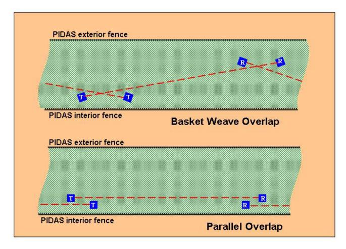
Figure 25: Active infrared sector intersection methods.
