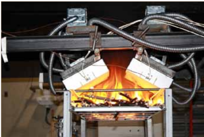
Figure 7.9 Radiant panel cable tray fire test (Side view of burning cables in a tray exposed to a radiant heat source)
