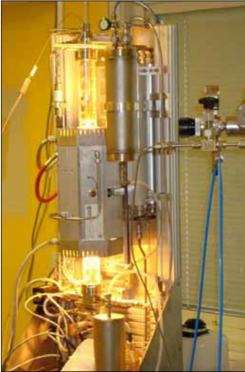
Figure 2.15 Integral LOCA test equipment operating at 1,200C, at Studsvik laboratory in Sweden, where tests will be conducted on high-burnup, irradiated fuel rods
