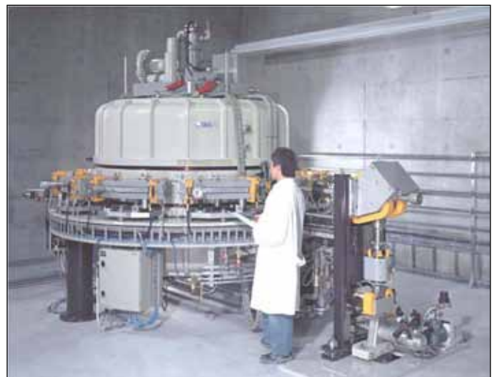
Figure 4.25 Rhodotron high-energy electron beam accelerator (Reference 1)
