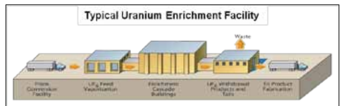
Figure 1.4 Typical uranium enrichment facility, part of the nuclear fuel cycle.
