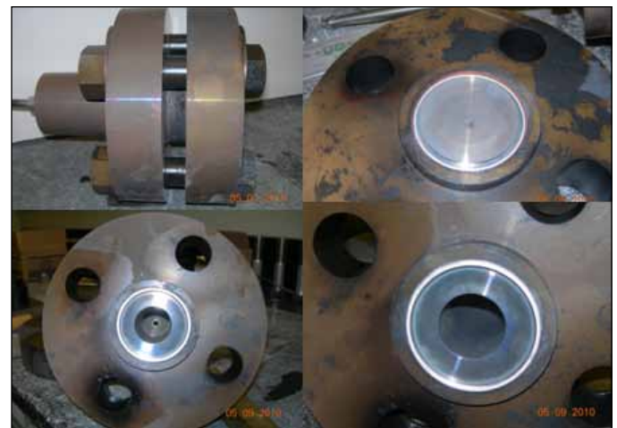
Figure 7.16 Pictures of the small-scale test vessel after 800°C exposure for 9 hours (small-scale test vessel (top left), vessel head after disassembly (top right), and vessel body and metallic seal after disassembly (bottom left and bottom right))
