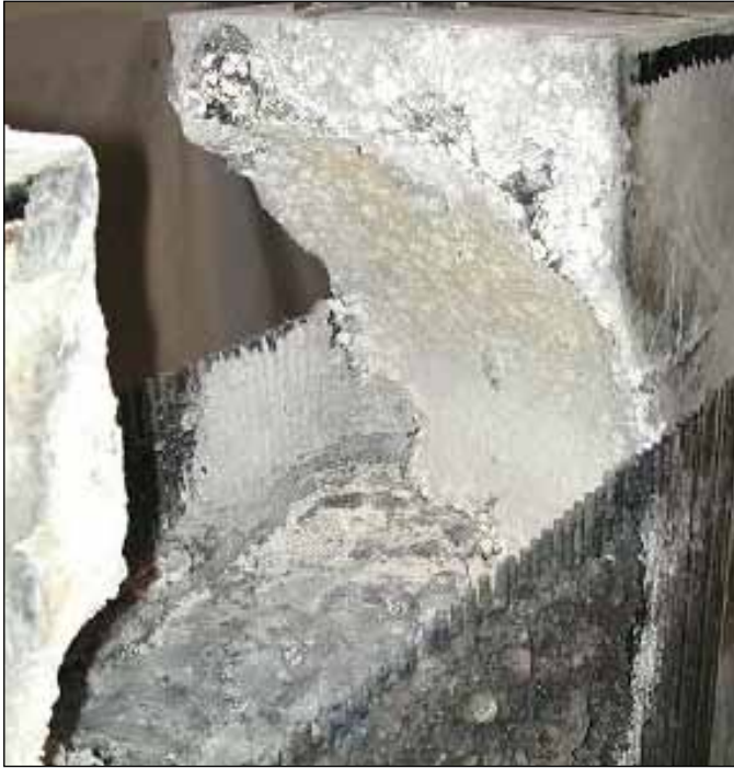
Figure 3.9 Posttest debris from CCI tests
