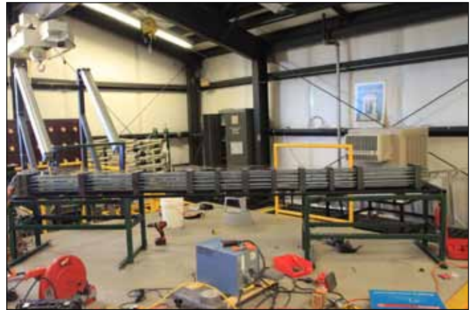
Single zirconium fuel assembly under construction prior to fire testing.
