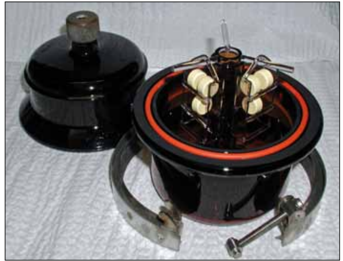
Figure 3.15 BIP irradiation vessel with sample coupons
