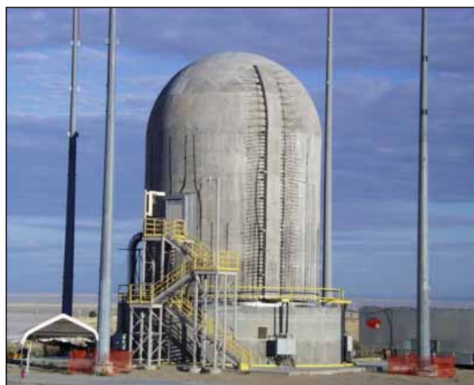
Figure 12.10 Completed prestressed concrete containment vessel ¼-scale model at SNL
