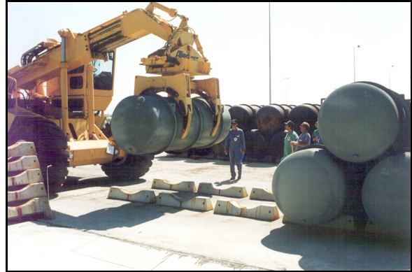
Figure 2-4 Stacking Depleted UF 6 Cylinders in a Storage Yard (DOE, undated a)
