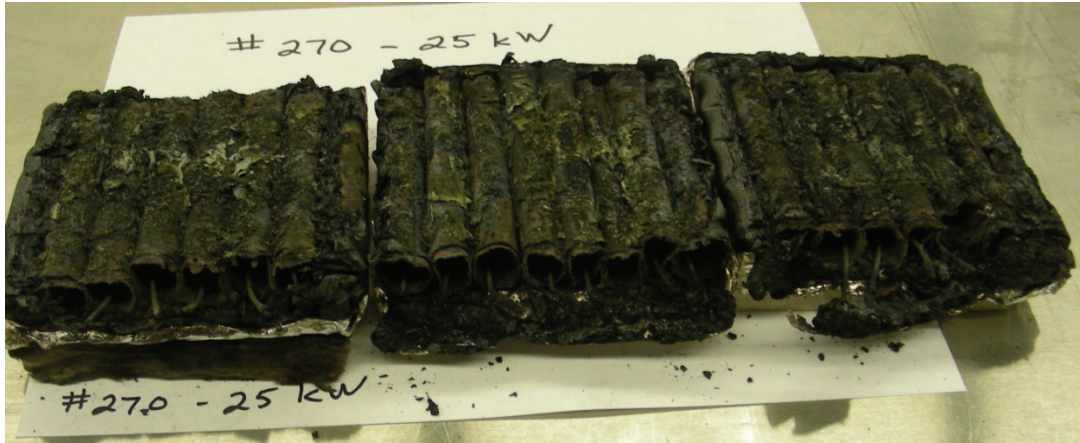
Figure 6-29. Photograph of Cable #270 after Cone Calorimeter test at 25 kW/m 2 .
