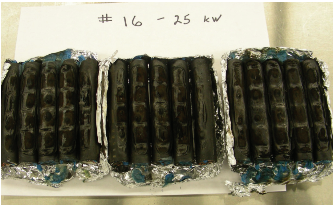
Figure 6-11. Photograph of Cable #16 after Cone Calorimeter test at 25 kW/m 2 .
