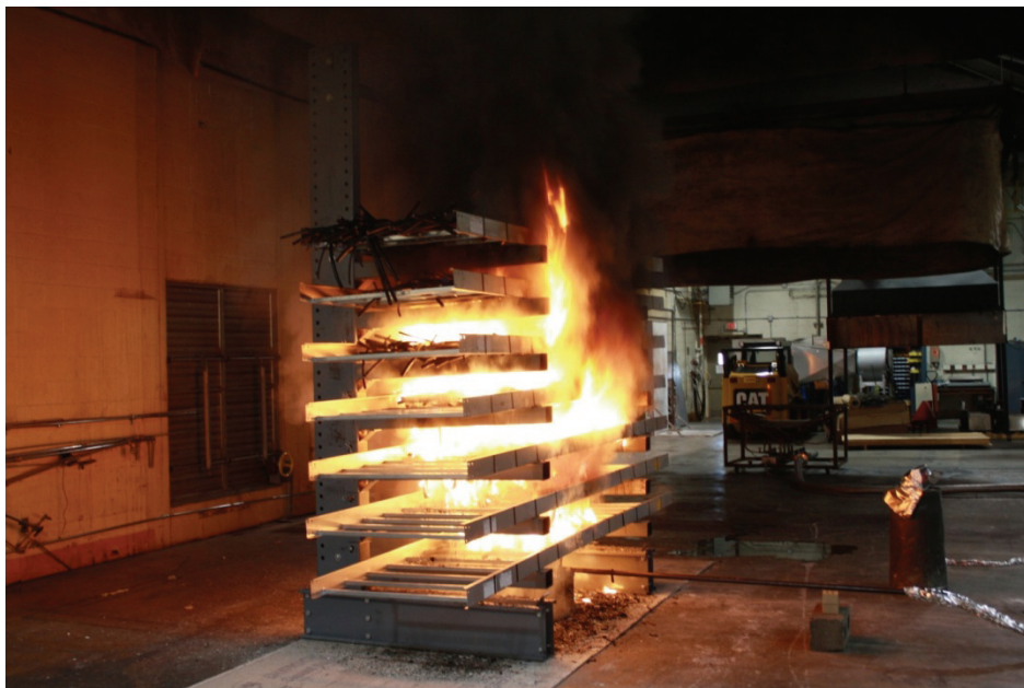
Figure 8-23. Multiple Tray Test 18 after approximately 20 min.
