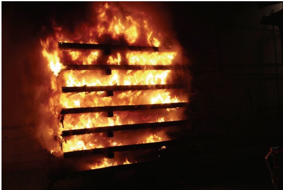
Figure 8-29. Photograph of Multiple Tray Test MT-22.
