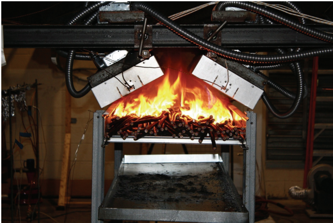
Figure 7-18. Photograph of RP Test 1, showing a relatively heavy load of cable.
