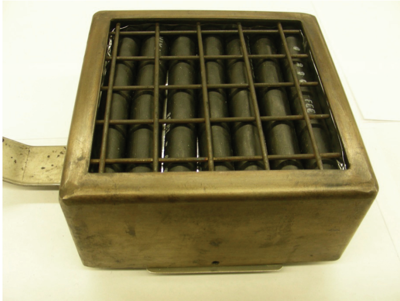
Figure 6-5. The completed holder assembly for the Cone Calorimeter.
