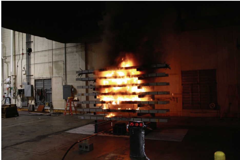
Figure 8-22. Multiple Tray Test 17 after 25 min.
