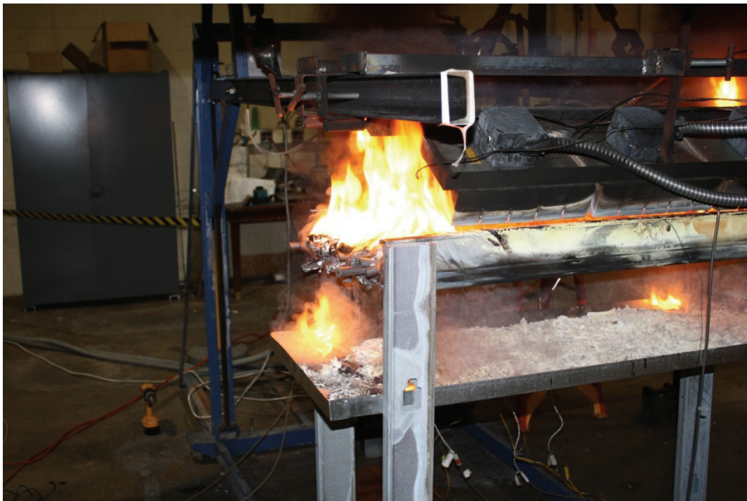
Figure 7-16. Photograph of RP Test 11 showing burning to the end of the tray.
