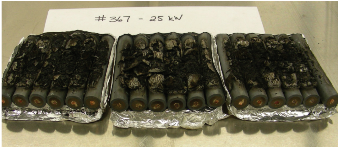
Figure 6-35. Photograph of Cable #367 after Cone Calorimeter test at 25 kW/m 2 .
