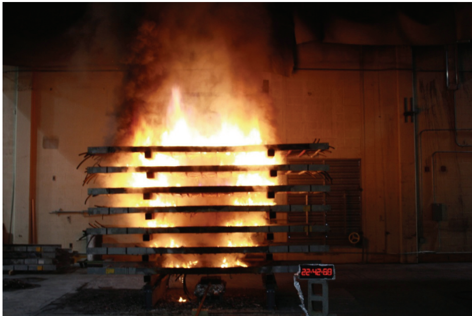
Figure 8-26. Photograph of Multiple Tray Test MT-20.
