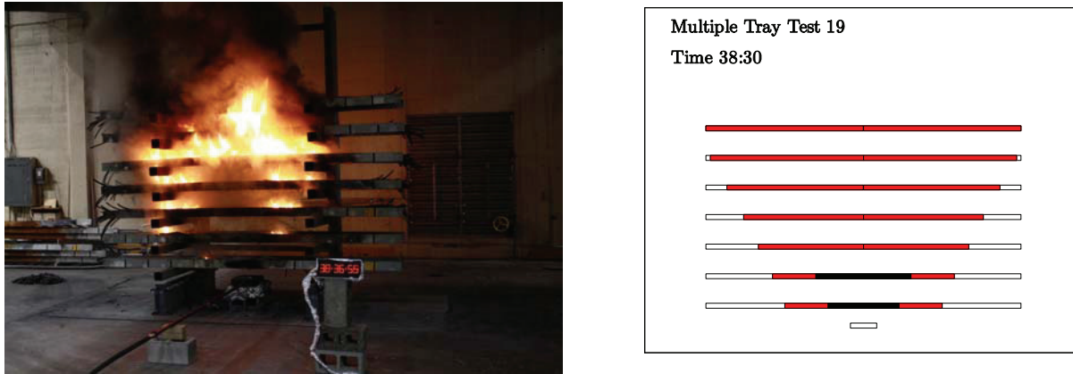
Figure 9-14. Photograph of MT-19 compared to the FLASH-CAT model prediction.
