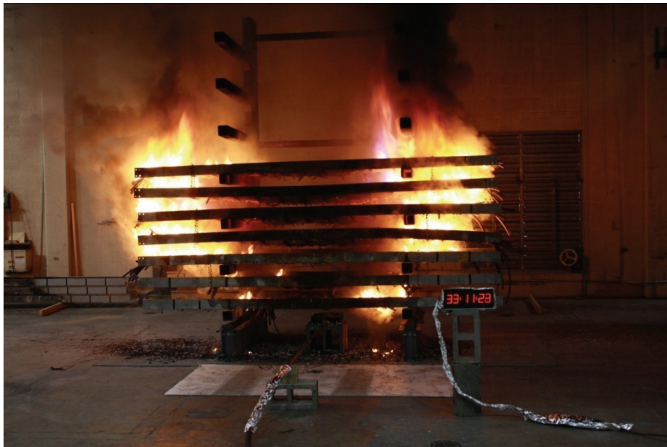
Figure 8-32. Photograph of Multiple Tray Test MT-24.
