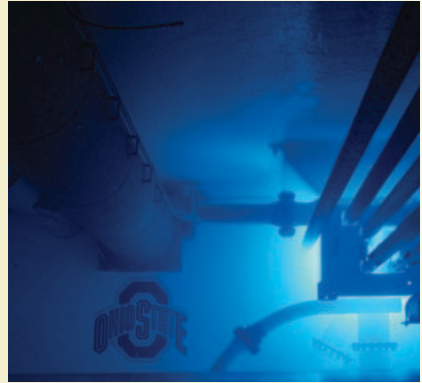
A blue glow of radiation, known as the “Cerenkov effect,” from nuclear fuel in the Ohio State Research/Test Reactor.
