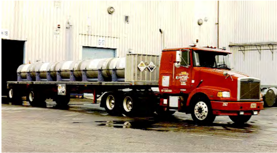
1 2 Figure 2-7 Truck Loaded with Five 30B Enriched Product Cylinders 3 Loaded for Transport in Their Protective Overpacks 4 (DOE, undated b) 5
