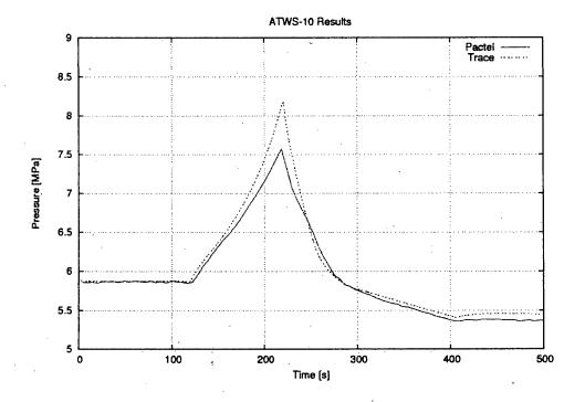
Figure 5. Pressure during the ATWS-10 transient.
