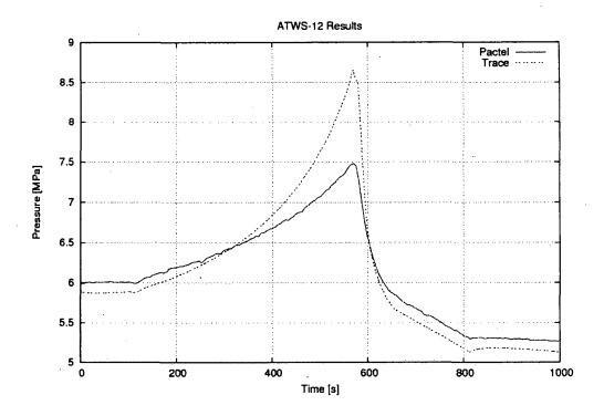
Figure 7. Pressure during the ATWS-12 transient.
