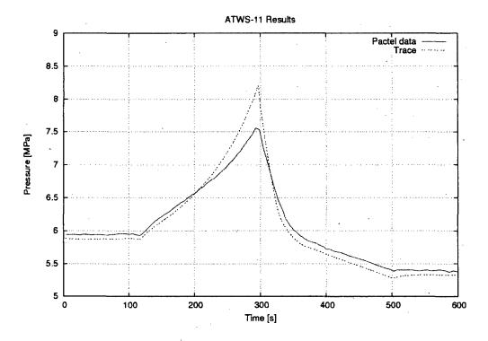
Figure 6. Pressure during the ATWS-11 transient.
