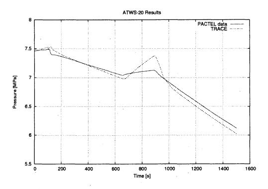
Figure 9. Pressure during the ATWS-20 transient.
