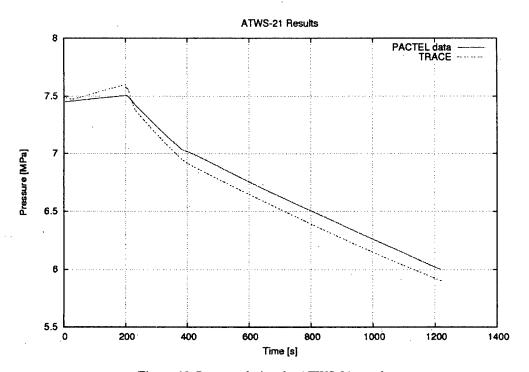
Figure 10. Pressure during the ATWS-21 transient.
