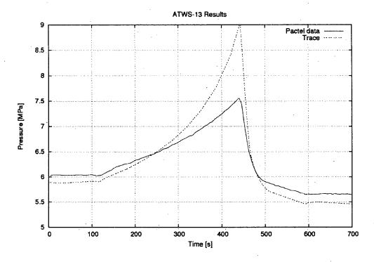
Figure 8. Pressure during the ATWS-13 transient.
