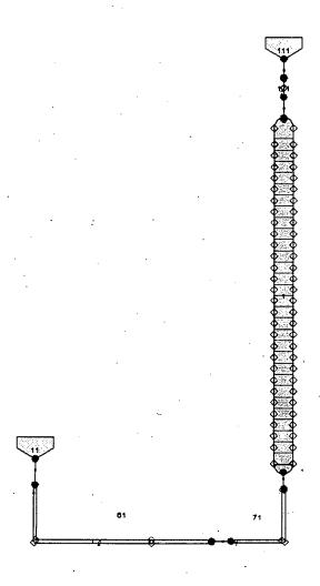
Figure 4. SNAP schematic of the PACTEL pressurizer including the FILL for surge line injection (11), the surge line and the FILL for spray (111). The width-length ratio of the PRIZER is 2:1.
