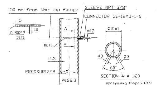
Figure 3. PACTEL pressurizer spray nozzle (Tuunanen et al., 1998).
