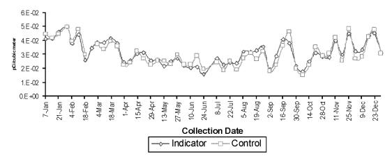
Figure 3 - Fermi 2 Air Particulate Gross Beta for 2009; the concentration of beta emitting radionuclides in airborne particulates samples was essentially identical at indicator and control locations. Gross beta activity varies throughout the year and is primarily an effect of seasonal precipitation.
