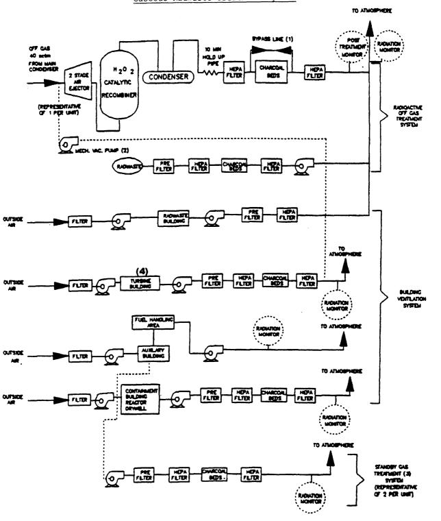
Figure 2.5-1 Gaseous Radwaste Treatment System
