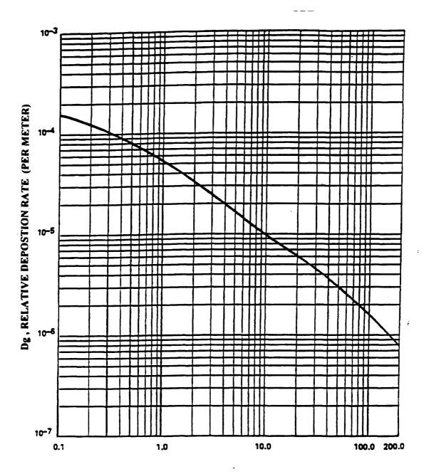
Figure 2.3-3 Relative Deposition for Ground-Level Releases (All Atmospheric Stability Classes)
